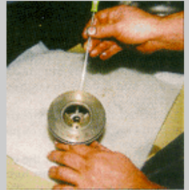
Fig. 5: Trapped carbon/oil deposits.
