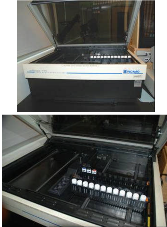
Figure 44 Commercial LSC counter (top) and detail of trays with vials (bottom)
