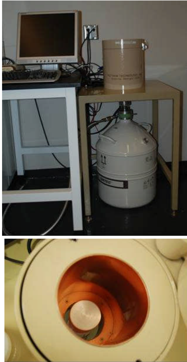
Figure 34 Commercial HPGe system (top) and detail of lead castle (bottom)
