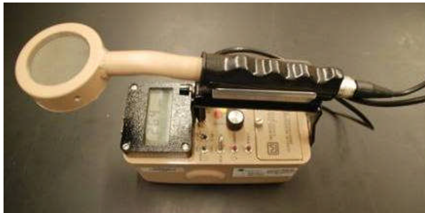
Figure 35 Portable contamination meter with pancake probe
