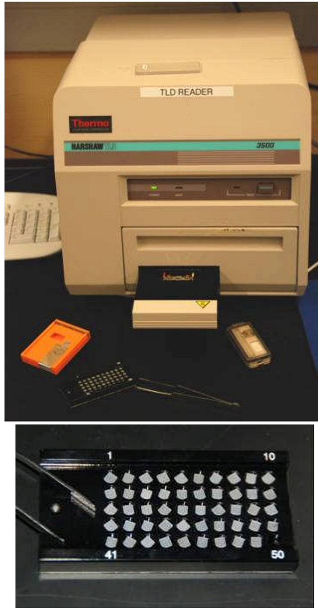
Figure 41 Commercial TLD reader (top) and tray of LiF chips (bottom)
