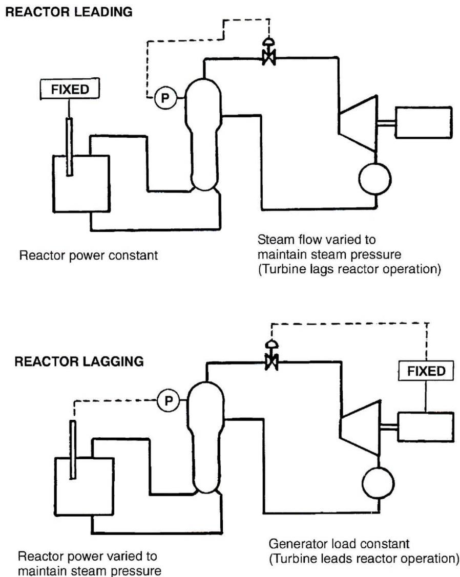
**Figure 1 Lagging and leading plant operation**
