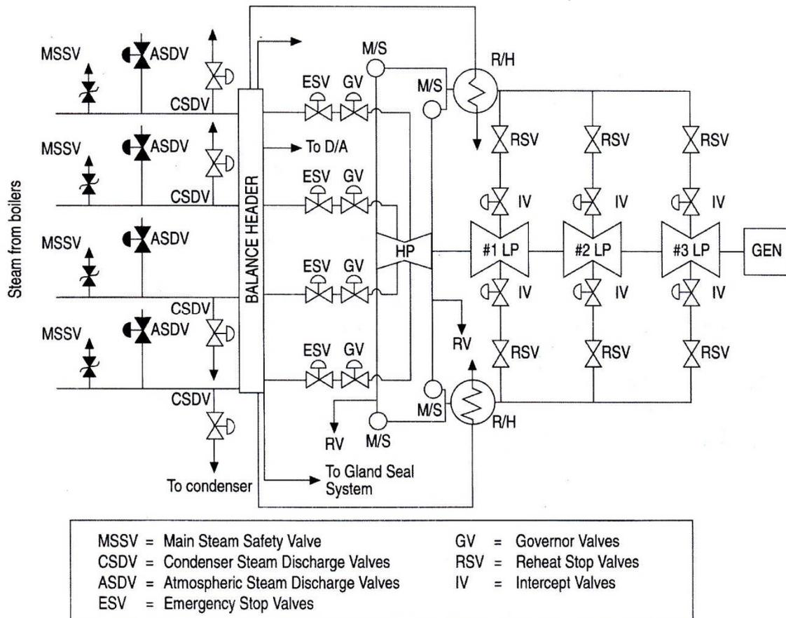
**Figure 16 Main steam system (Point Lepreau) (courtesy of NB Power)**
