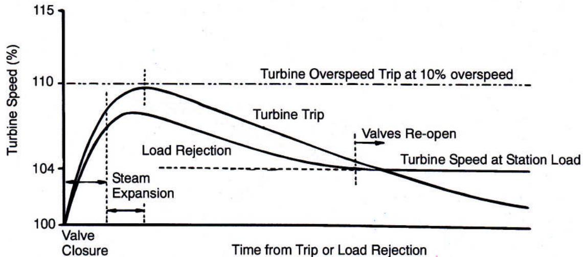
Figure 35 Turbine-generator load rejection
