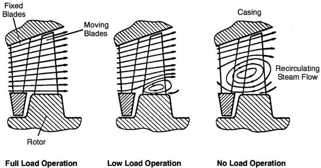
**Figure 32 Recirculation of steam at low loads (courtesy of NB Power)**
