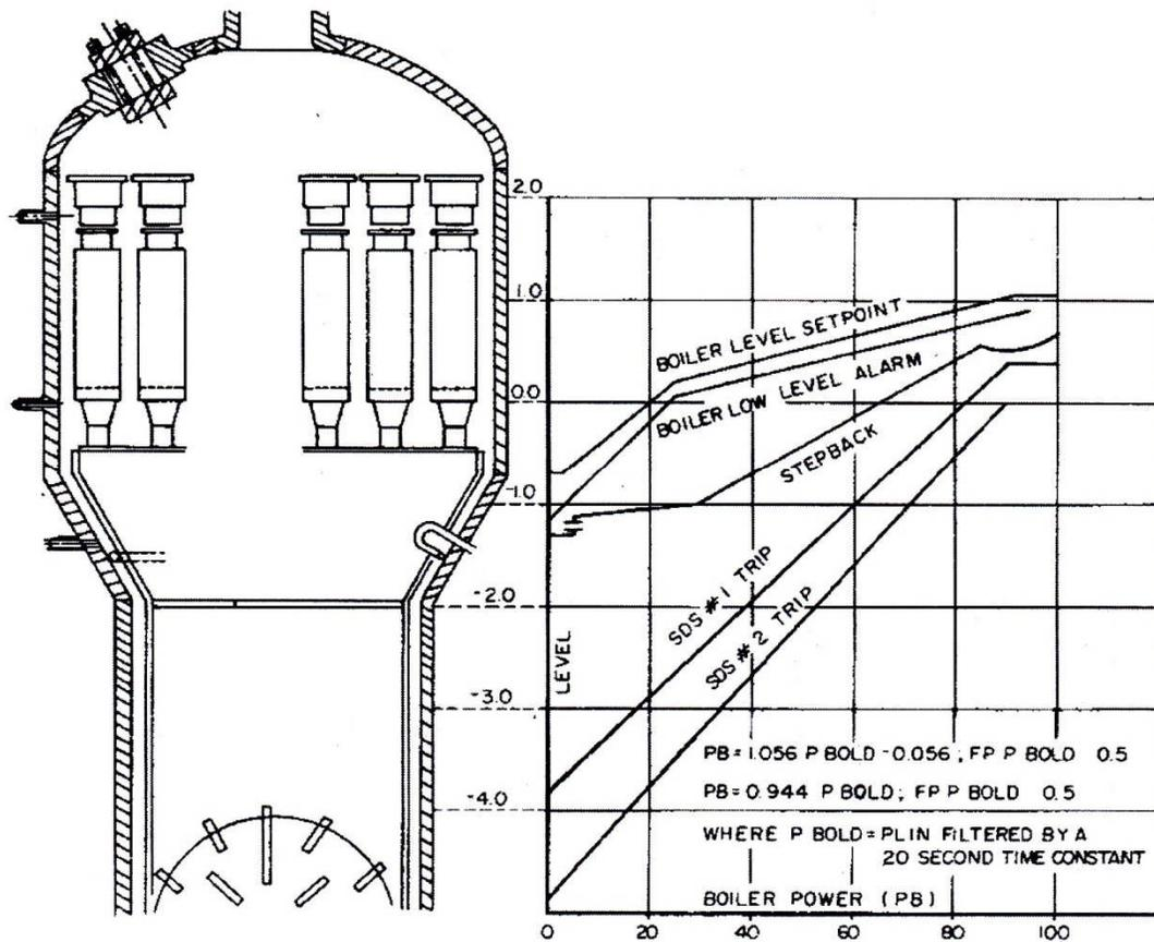
Figure 15 Steam generator level alarms and set points (courtesy of NB Power)
