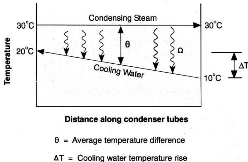
**Figure 17 Condenser temperature profile**
