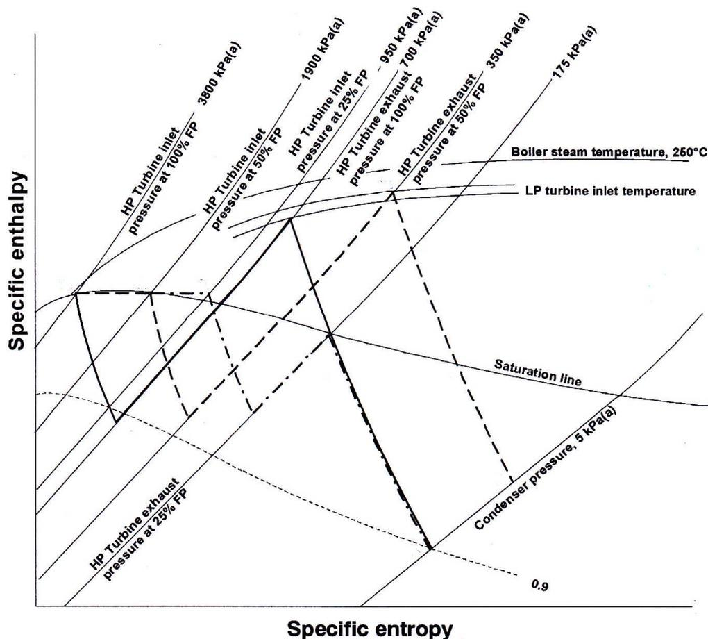
**Figure 30 Partial load turbine expansion lines (courtesy of NB Power)**
