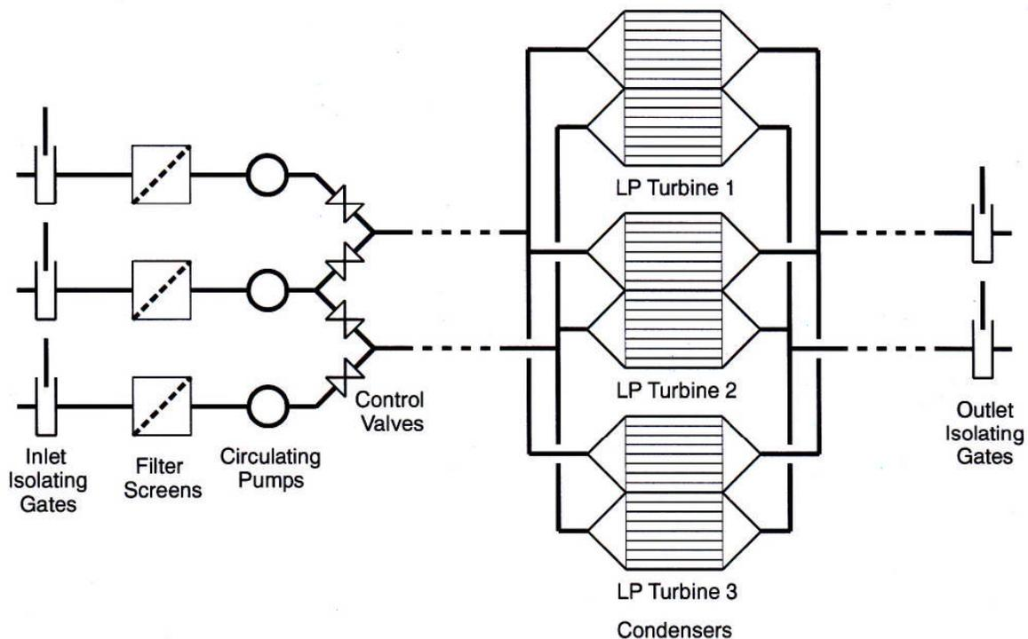
**Figure 21 Typical condenser cooling water system**
