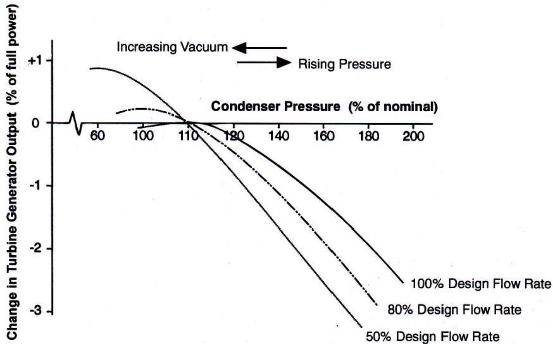
**Figure 23 Effect of change in condenser pressure (courtesy of NB Power)**
