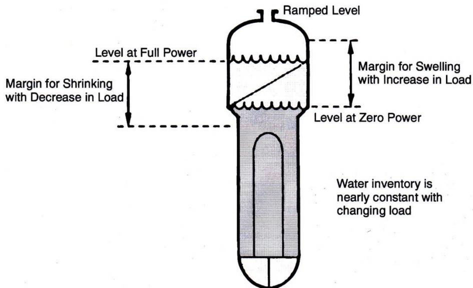
**Figure 13 Ramped steam generator water level**
