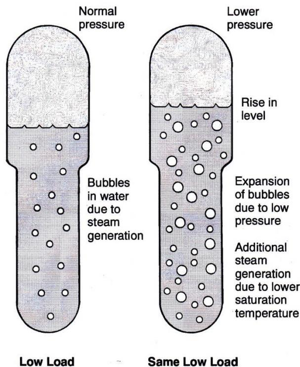
**Figure 11 Transient swelling due to changing load conditions**
