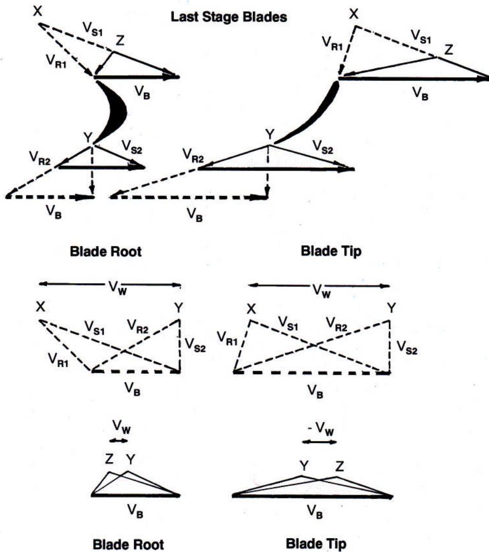
Figure 31 Change in whirl velocity at low loads
