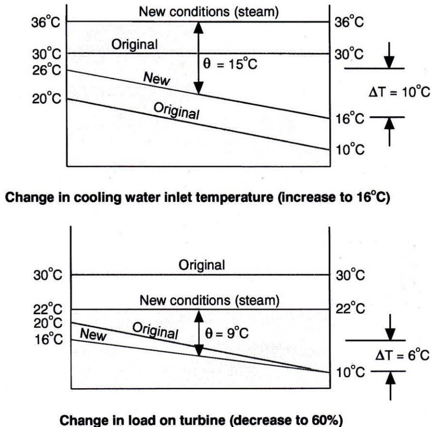
**Figure 18 Changes in condenser temperature profile**
