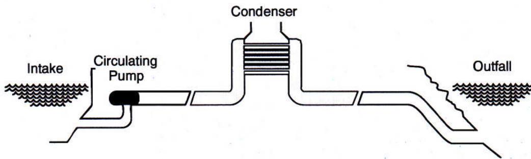
**Figure 22 Simplified condenser cooling water system**
