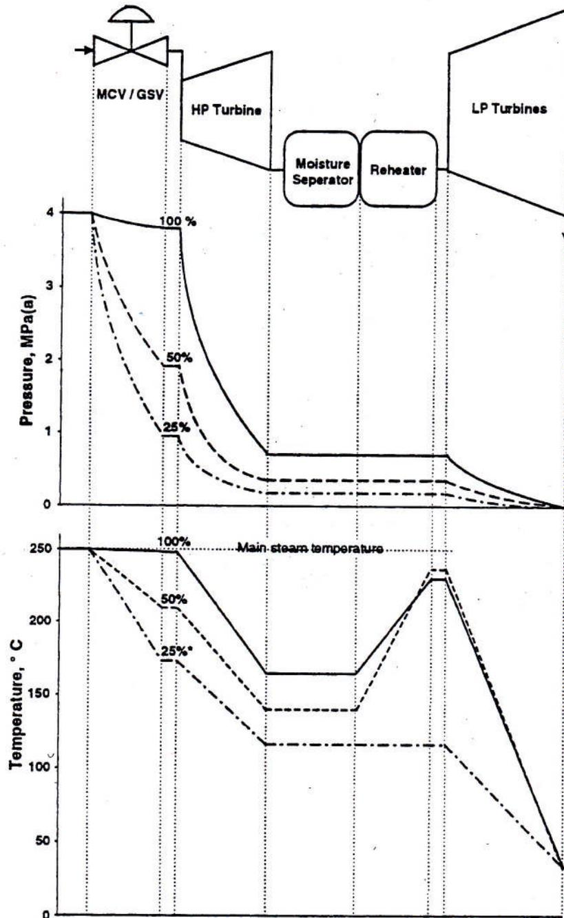
Figure 27 Steam pressure variation through the turbine (courtesy of NB Power)
