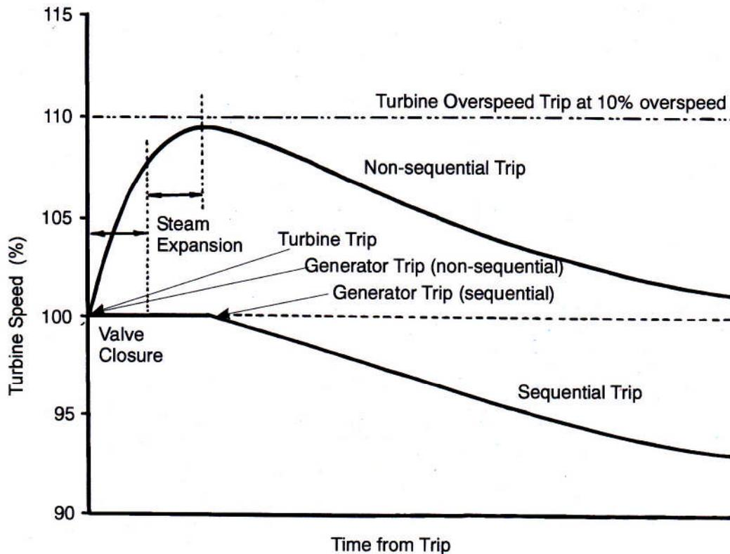
**Figure 34 Turbine generator non-sequential and sequential trips**
