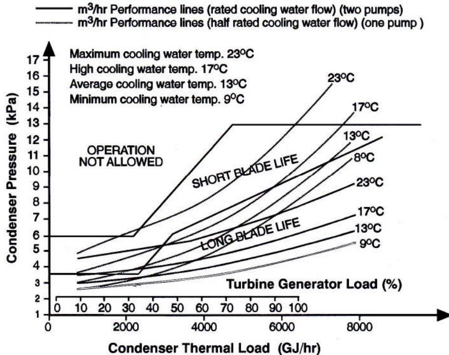
Figure 20 Condenser performance curves (adapted courtesy of Eskom)
