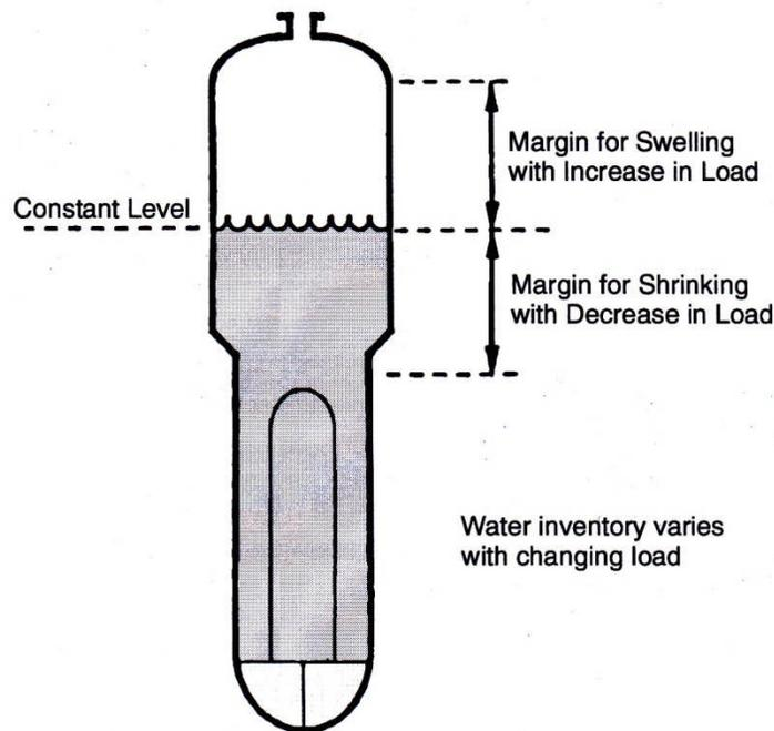
**Figure 12 Constant steam generator water level**
