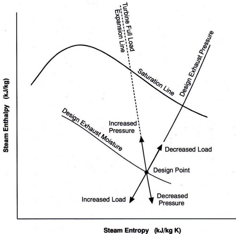
Figure 24 Effect of change in turbine load and condenser pressure
