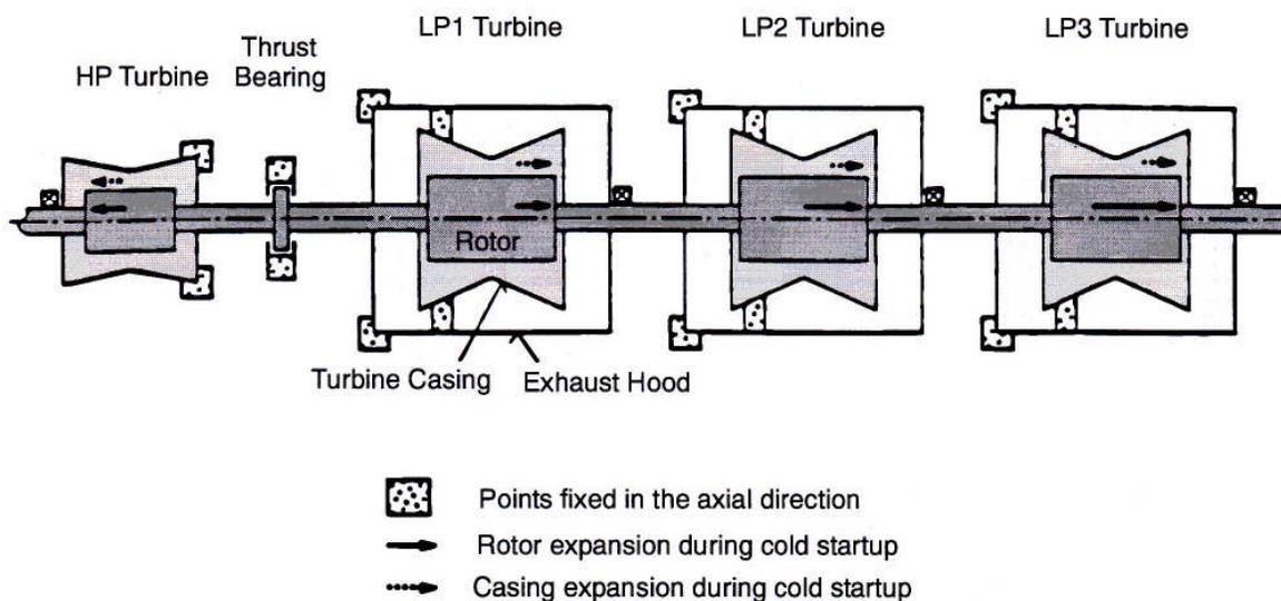
**Figure 33 Differential axial expansion of turbine rotors and casings**
