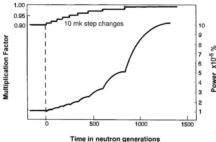
**Figure 4 Stabilization time for different subcritical multiplication factors**
