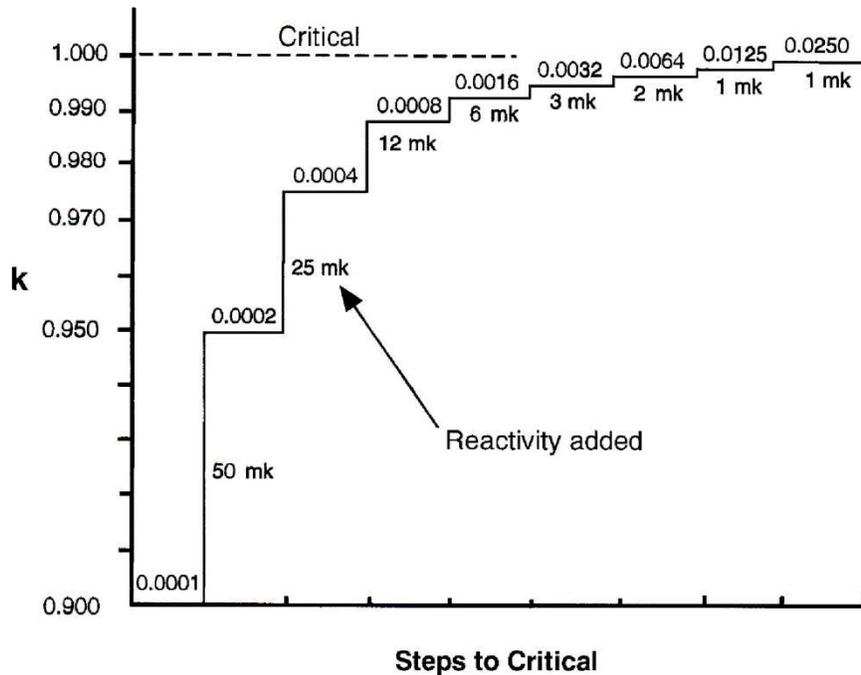
**Figure 5 Approach to critical - subcritical multiplication factor change**
