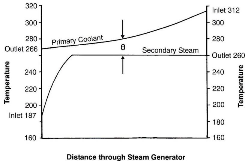
**Figure 9 Steam generator temperature profile**
