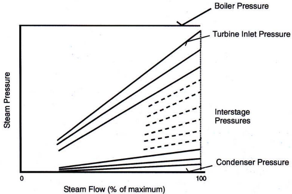
Figure 28 Steam pressure variation with load change
