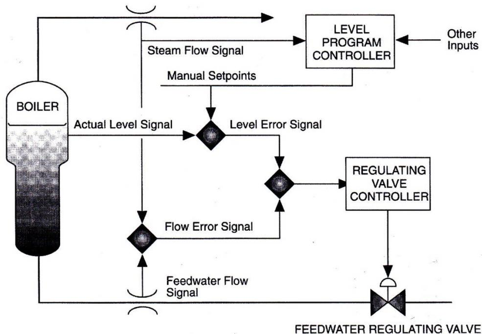
**Figure 14 Three element steam generator level control system
