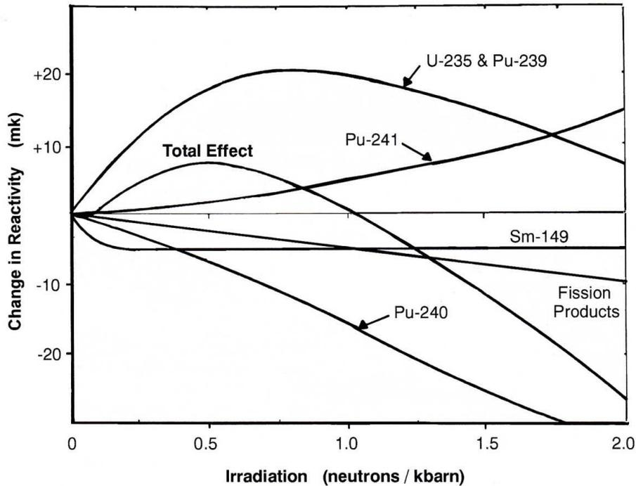
Figure 8 Effects of fuel burnup on reactivity
