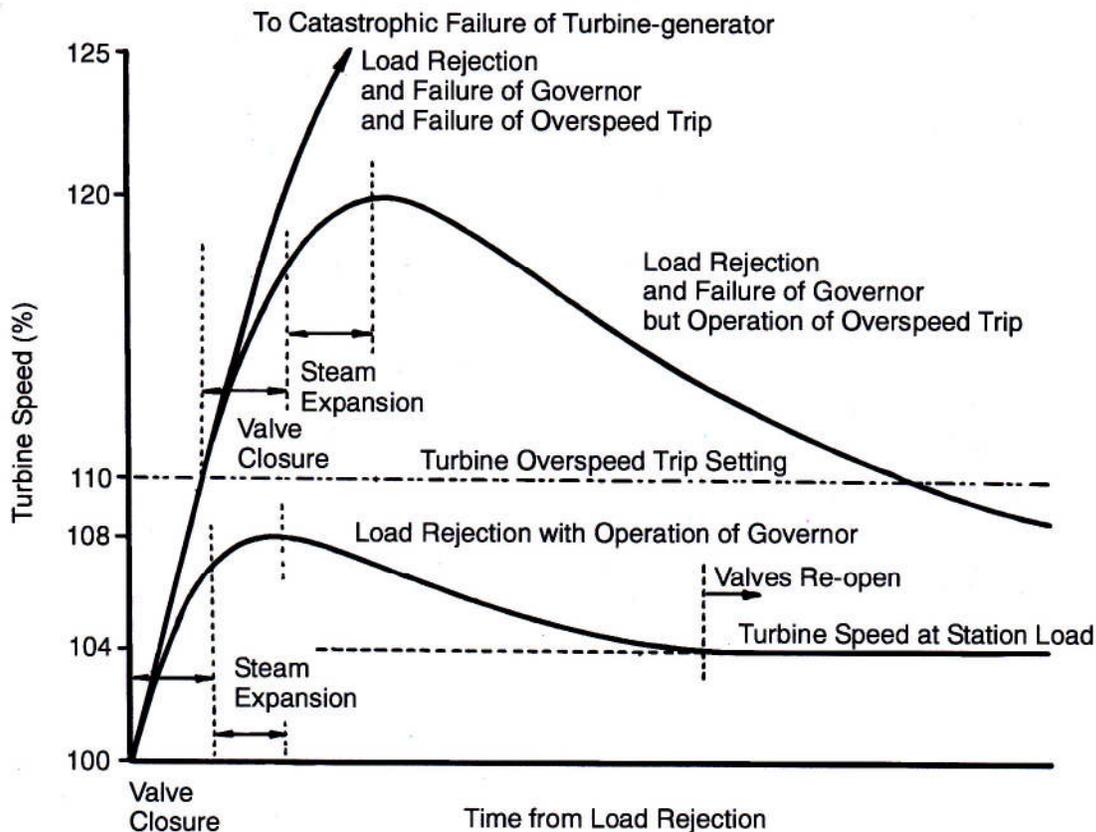
Figure 36 Turbine generator overspeed trip
