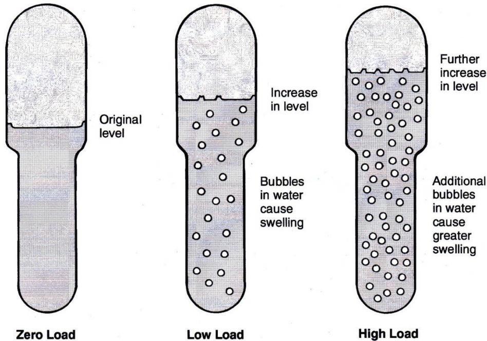
**Figure 10 Steady state swelling due to different load conditions**
