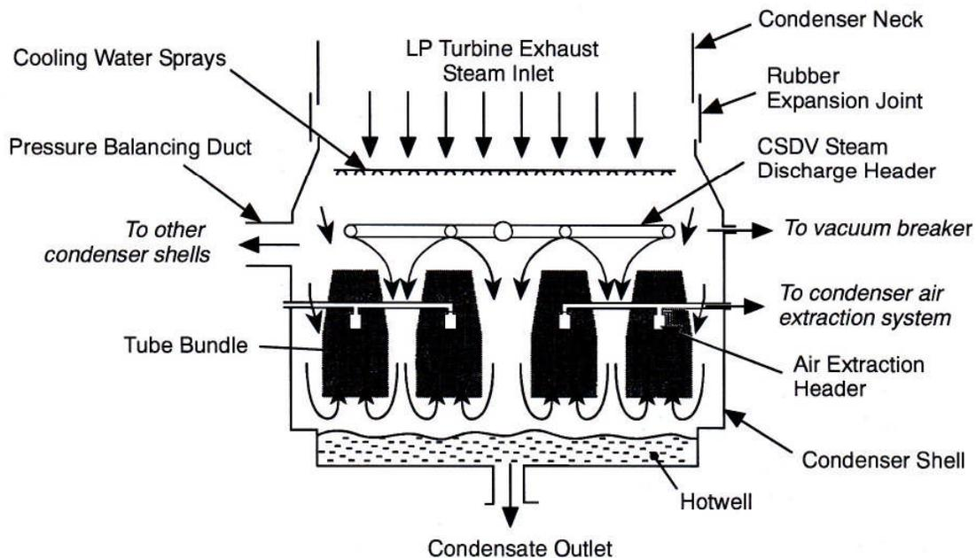
Figure 25 Condenser cross section (courtesy of NB Power)
