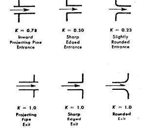
Problem: Determine the total resistance coefficient for a pipe one diameter long having a sharp edged entrance and a sharp edged exit.
