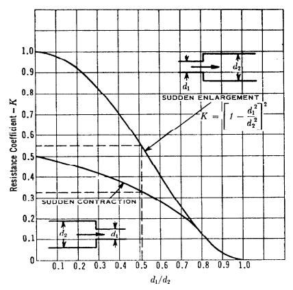
Sudden enlargement: The resistance coefficient K for a sudden enlargement from 6-inch Schedule 40 pipe to 12-inch Schedule 40 pipe is 0.55, based on the 6-inch pipe size.
