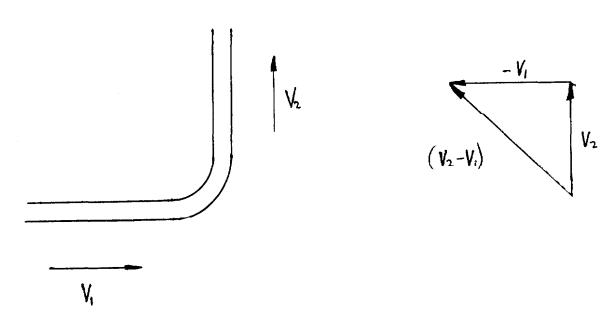
The change in velocity =  $V_2-V_1$ .  $(V_2-V_1)$  is the direction in which the force has to be applied to prevent the pipework moving.
