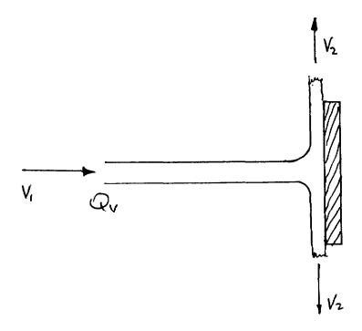
Consider a jet striking a flat plate. The final velocity of the fluid is at 90° to the original velocity and the jet is split in radial directions, thus  $V_2$  is zero. Thus the change in velocity =  $V_2-V_1=0-V_1$ . Thus the force exerted by the plate, to deflect the jet, has to act in the opposite direction to the flow.
