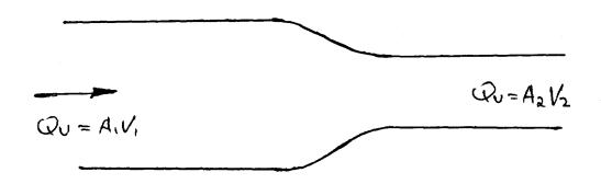
Force on nozzle =  $\ell \times Q_V \times (V_2-V_1)$
