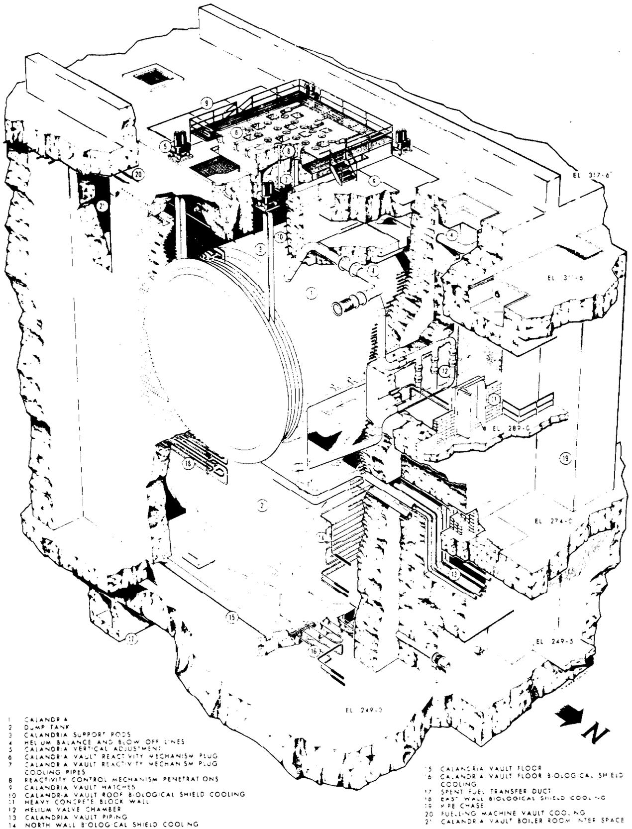
Figure 6: Water Cooled Heavy Concrete Biological Shielding PGSA (NPD and Douglas Point are similar)
