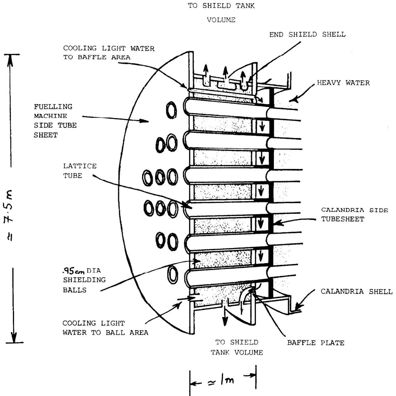
Figure 5: END SHIELD-SHIELD TANK COOLING (BRUCE GSA)
