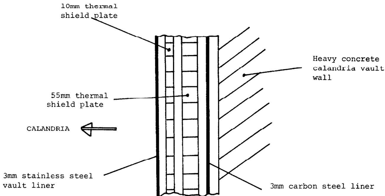
Figure 2: Typical Douglas Point Thermal Shield
