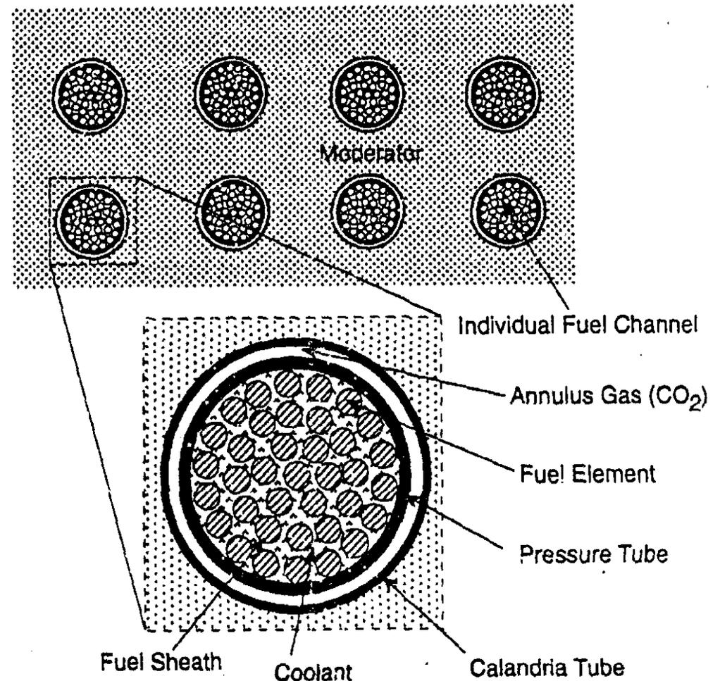
Figure 3-1: Arrangement of fuel channels & moderator.
