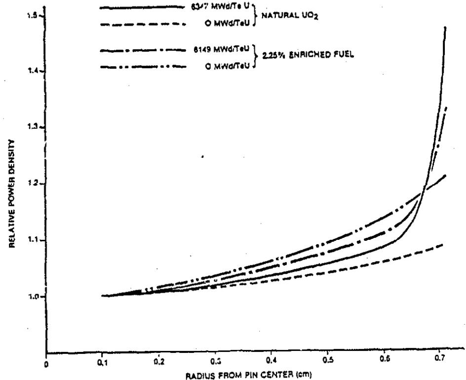
Figure 3-3: Power density distributions in UO<sub>2</sub> fuel pin.
