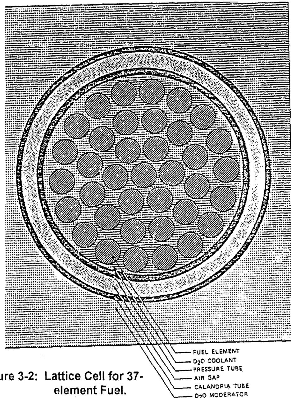
Figure 3-2: Lattice Cell for 37-element Fuel.
