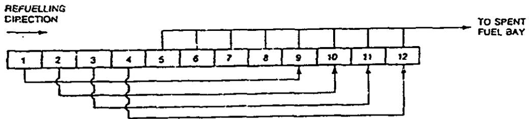
Figure 4.1 Standard 8-Bundle-Shift Refuelling Scheme
