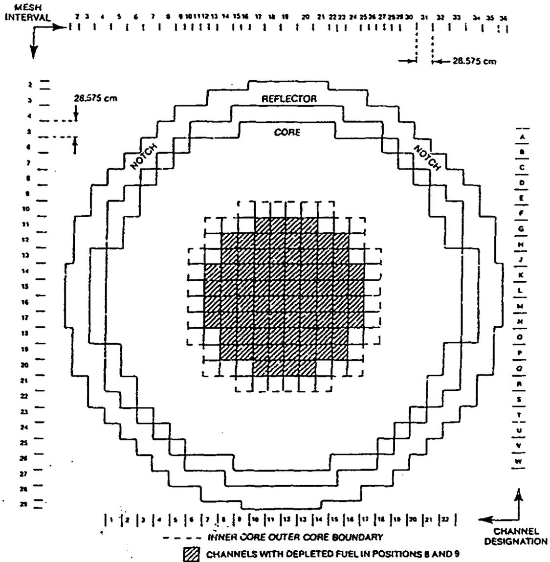
Figure 4.3 600 MW Reactor Model Face View Showing Initial Loading of Depleted Fuel
