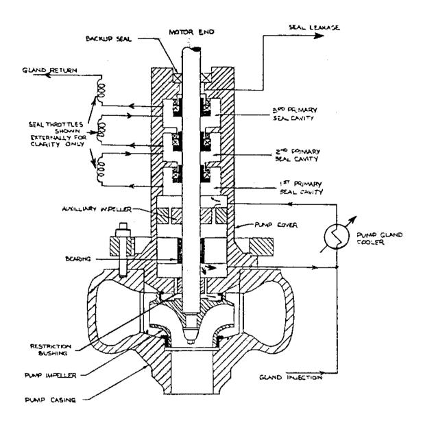
Figure 2: Simplified HT Pump Gland
