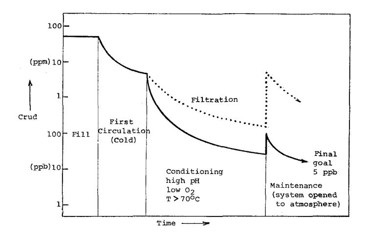
solid line - following chemical conditioning procedures dotted line - using filters to remove the crud
