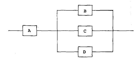
In the above system, a system failure consists of a failure of either component A, or a failure of at least two of B, C, D.
