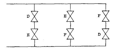
The above diagram is a schematic representation of the typical dump valve arrangement for a reactor with moderator dump. The opening and closing of valves D, E and F are controlled by channels D, E and F respectively. During five years of reactor operation, the electronics of channels D, E and F were tested three times a week and four unsafe failures of individual channels were found.
