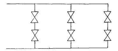
The above diagram is a schematic representation of the typical dump valve arrangement for a reactor with moderator dump. In five years of operation of this reactor, six failures (to open) of individual valves were found. The dump valves are tested twice a week.
