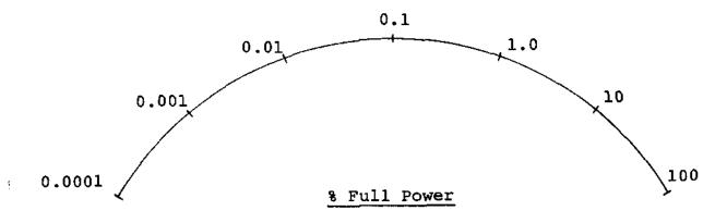
The above diagram represents the face of an instrument which indicates neutron power on a logarithmic scale. Given that 100 megawatts is 100% power, mark the positions on the scale which correspond to the following power levels:
