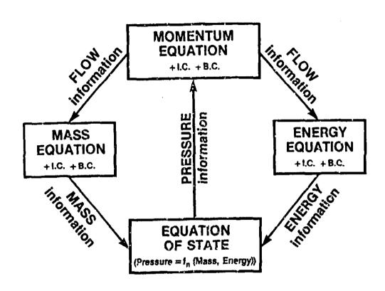
Figure 6.1 The four cornertone equations for thermalhydraulic system simulation and the flow of information between them.
