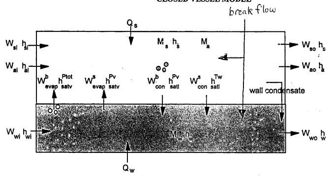
W h h Ptot enthalpy carried by flashing of liquid at surface
