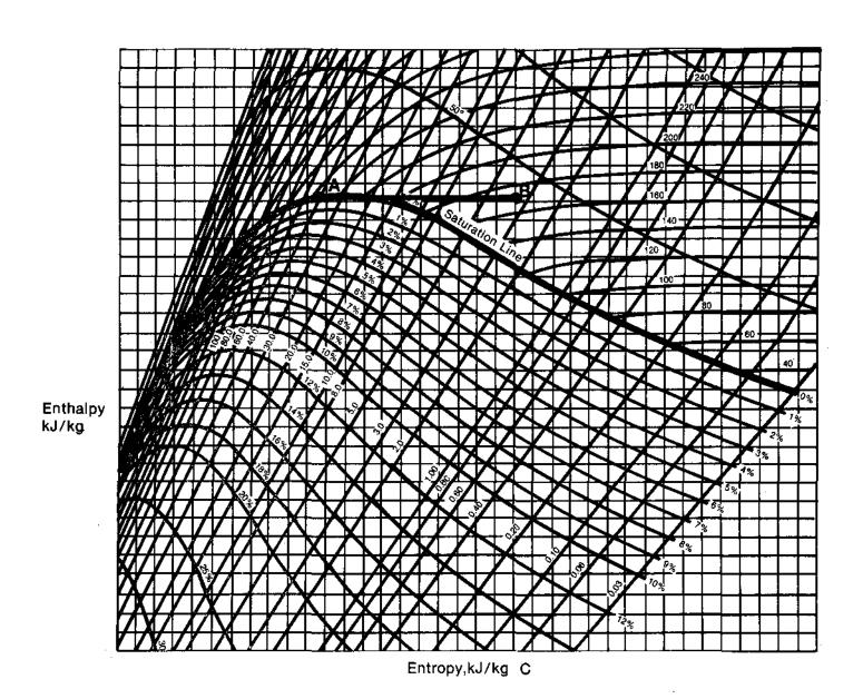
As the diagram shows, both the pressure and temperature of the steam are reduced, and it becomes superheated (zero moisture content).
