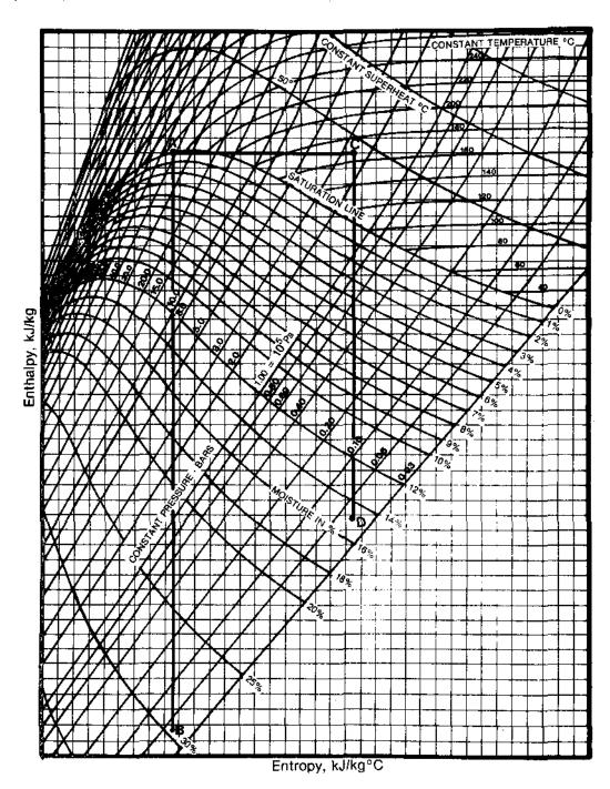
As the diagram shows, throttling of the steam supplied to the turbine reduces the amount of heat which can be converted into mechanical work by the turbine (h\_A - h\_B > h\_C - h\_D).
