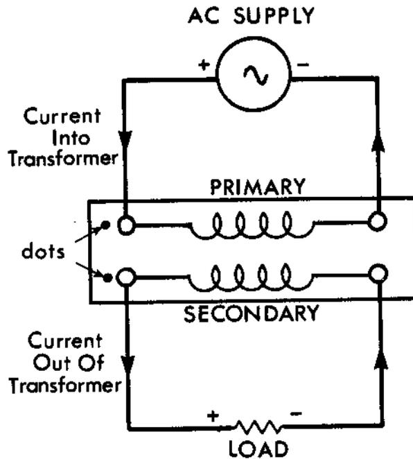
Figure 7: Polarities and Current Flows Associated with an ac Supply, Transformer and Load.
