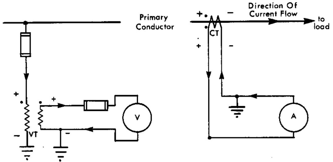
Figure 8(a): VT Supplying a Load.
