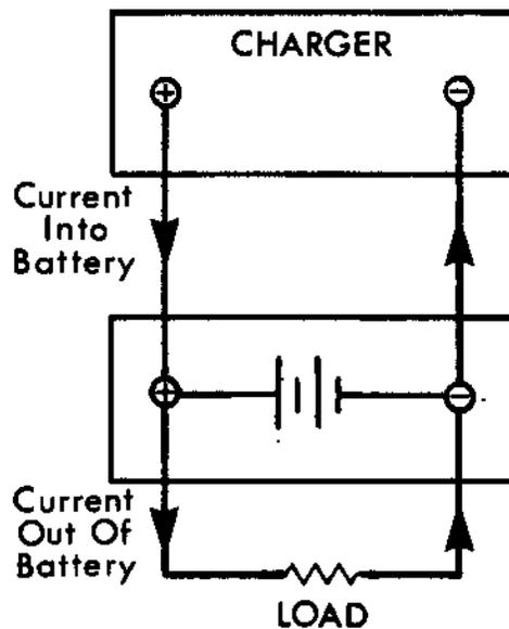
Figure 6: Polarities and Current Flows Associated with a Charger, Battery and Load.
