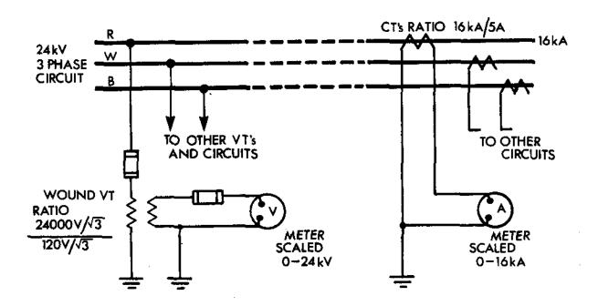
Figure 6: Voltage Measuring Figure 7: Current Measuring Circuit.
