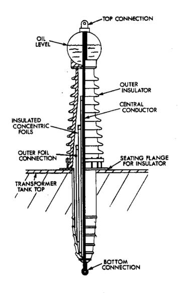
Figure 3: Half Section of a High Voltage Bushing.
