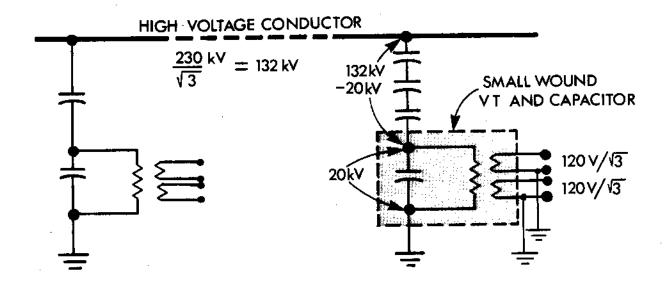
Figure 1: Symbol for a Capacitor Voltage Transformer.
