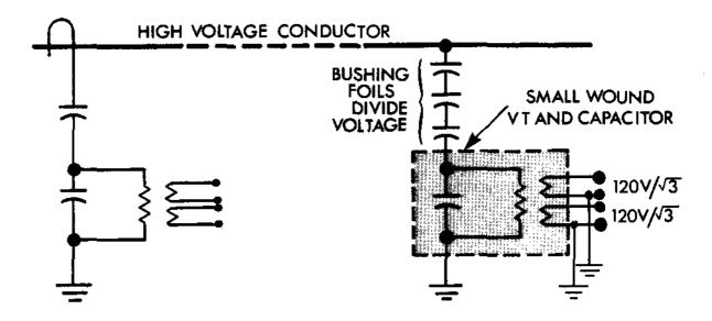
Figure 4: Symbol for a Bushing Capacitor Voltage Transformer.
