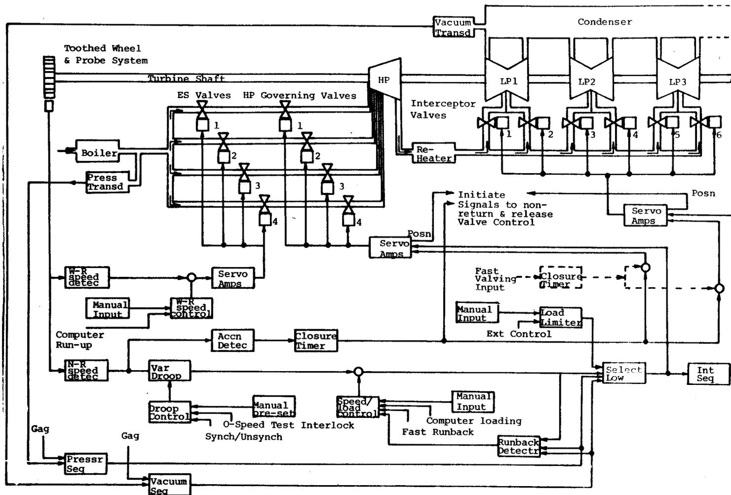
Block Diagram of Electrical-Hydraulic Governing System
