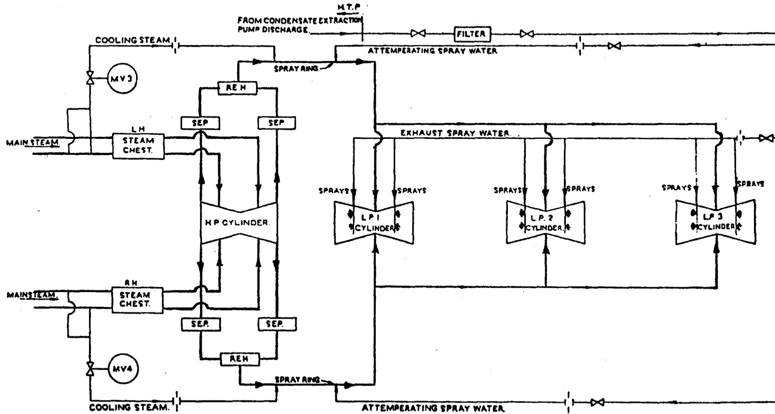
Schematic Arrangement of LP Cylinder Exhaust Spray Cooling System and Cooling Steam System
