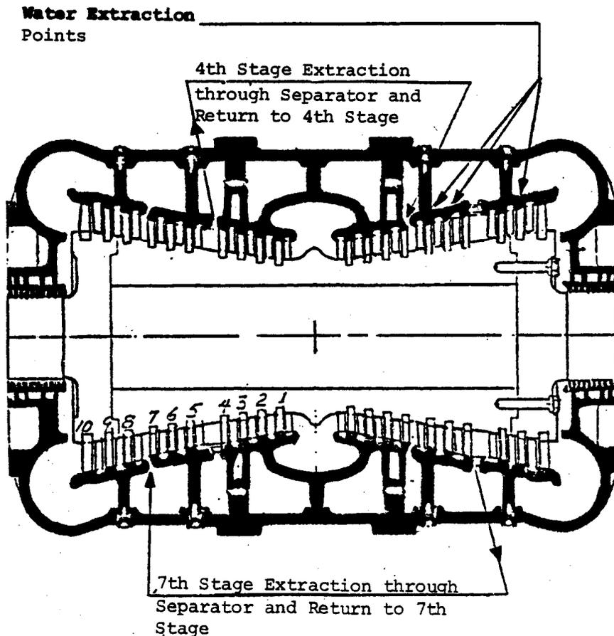
HP Turbine With Auxiliary Separators
