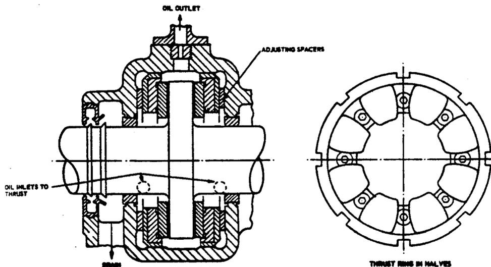
Tilting Shoe Thrust Bearing
