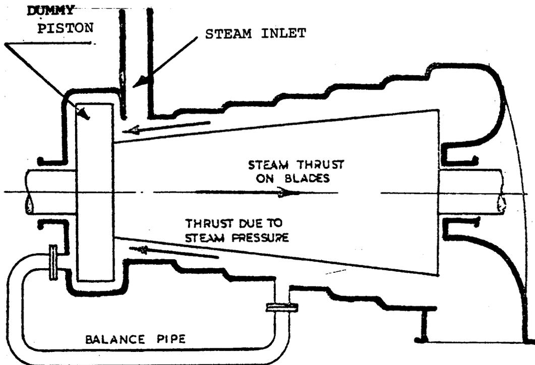
Single Flow Reaction Turbine with Dummy Piston
