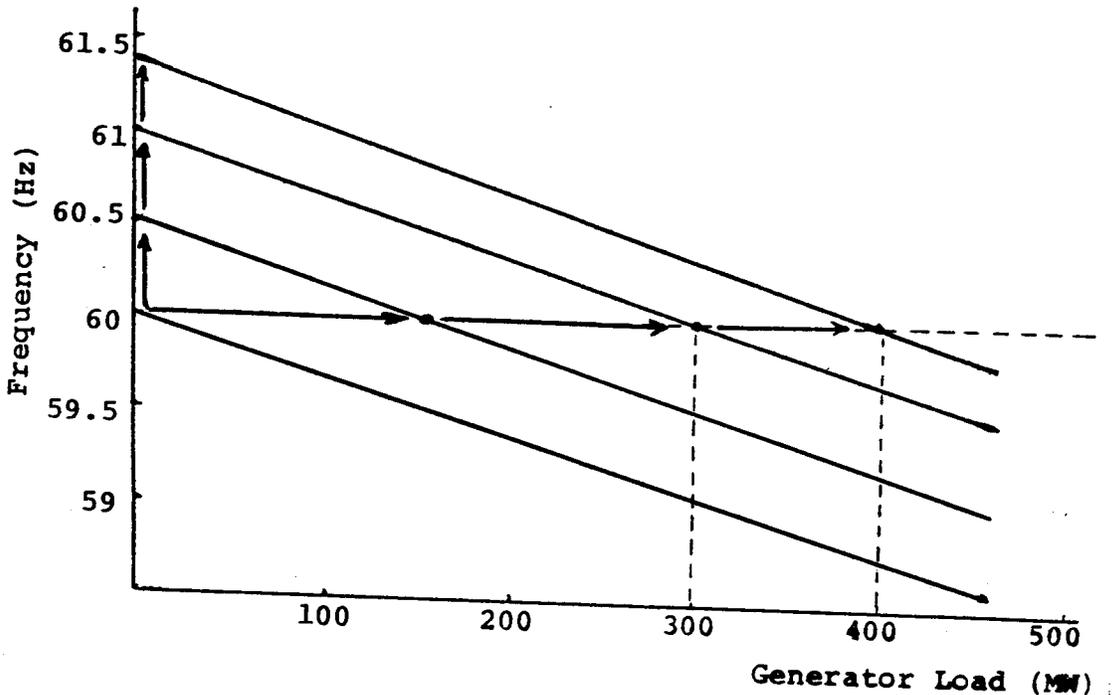
Increasing Load on a Synchronized Turbine/Generator
