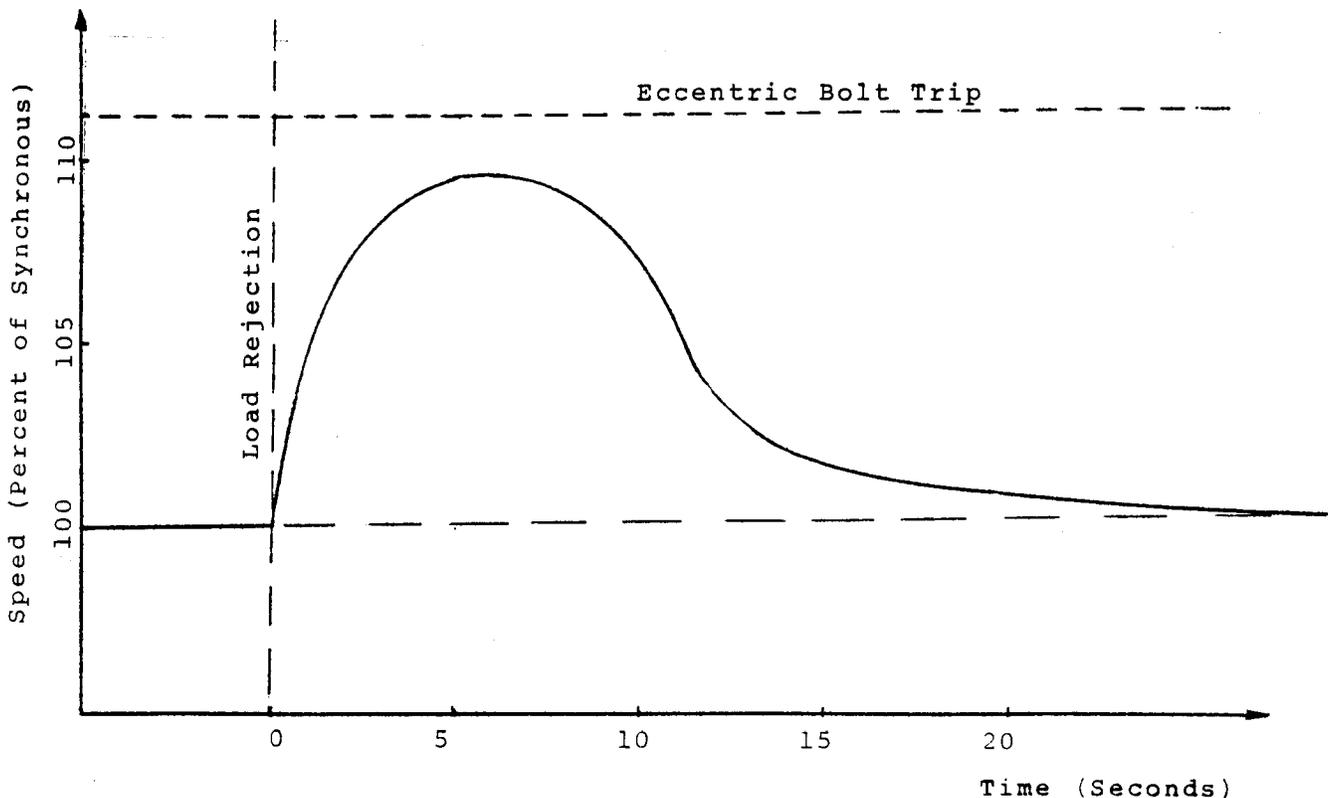
Electrical - Hydraulic Governing System on Load Rejection
