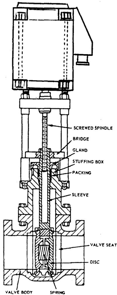
Steam Isolating Valve (Boiler Stop Valve)
