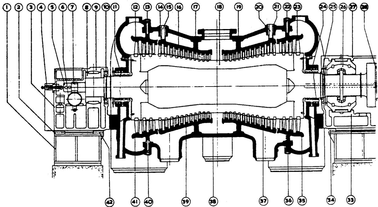
Typical HP Turbine with Extraction Steam after Stage 11
