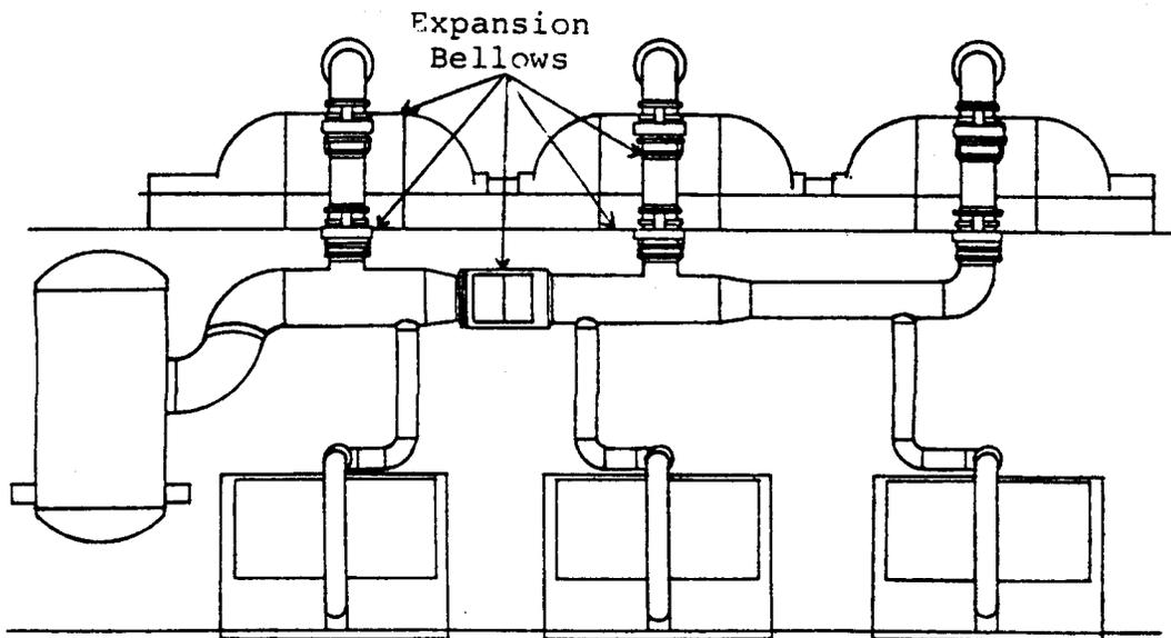
Expansion Joints on LP Turbine Inlet
