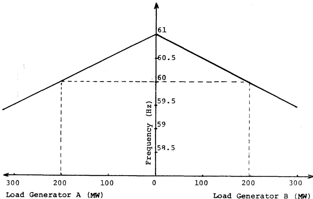
Two Turbine/Generator Sharing a 400 MW Load
