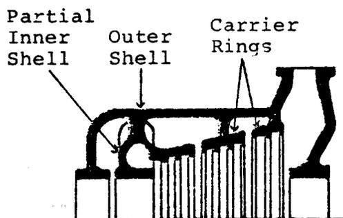
Single Flow Turbine with Carrier Rings
