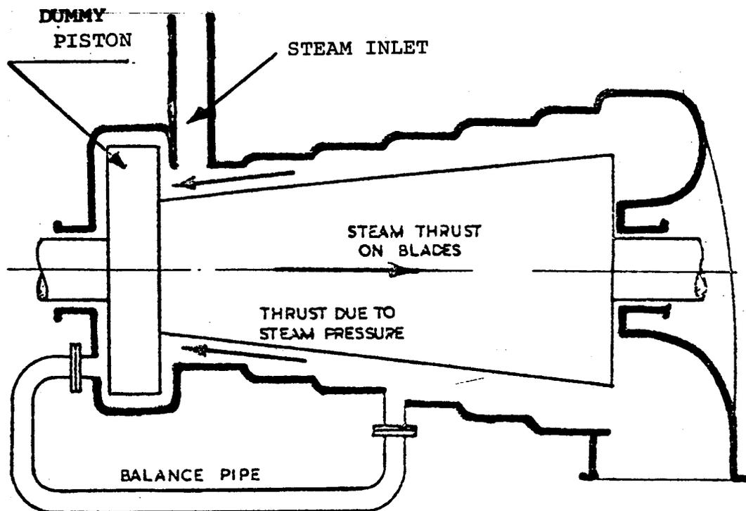
Single Flow Reaction Turbine with Dummy Piston
