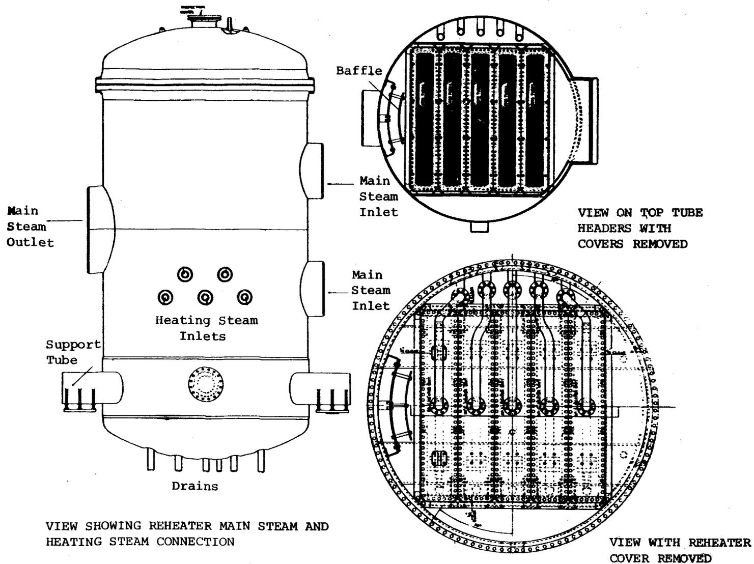
VIEW SHOWING REHEATER MAIN STEAM AND HEATING STEAM CONNECTION
