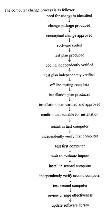
It has been found that identification of the exact nature of the proposed change is important. For example, one requested change asked for a program to recognize a reactor trip if two of three reactor trip signals were received. It did just that, and did not recognize three of three reactor trip signals as a reactor trip.
