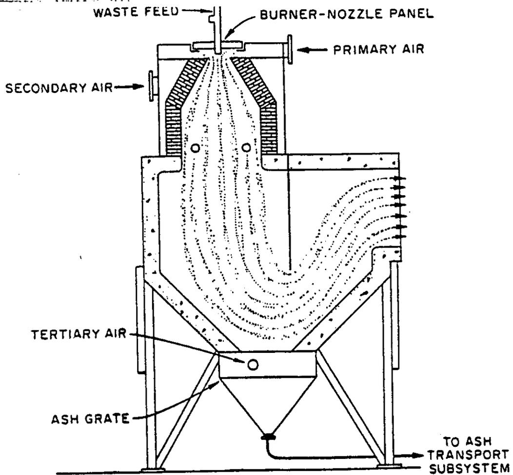
Figure 5-11 Excess-air cyclone incinerator combustion chamber. Source: (DOE 1984).
