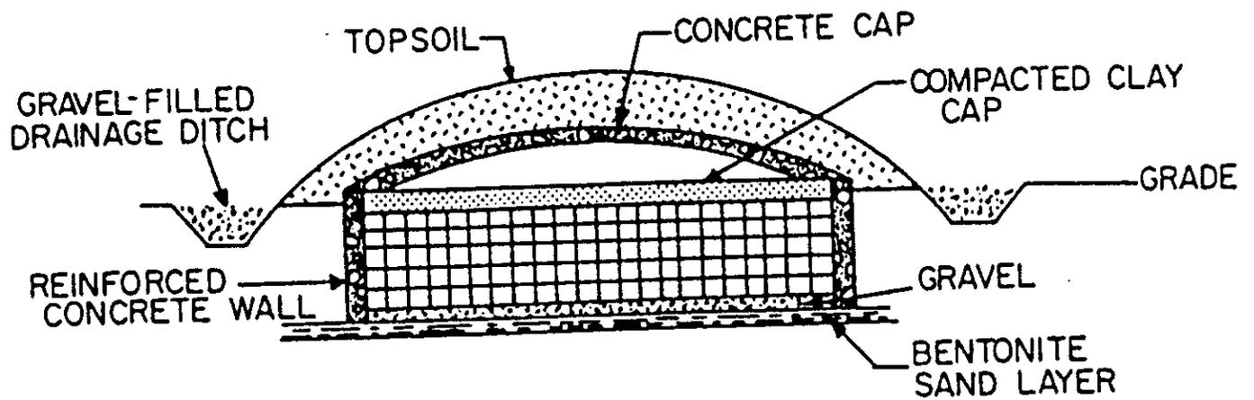
**Earth-mounded concrete bunker, developed by the French. (Courtesy of the U.S. Nuclear Regulatory Commission.)**
