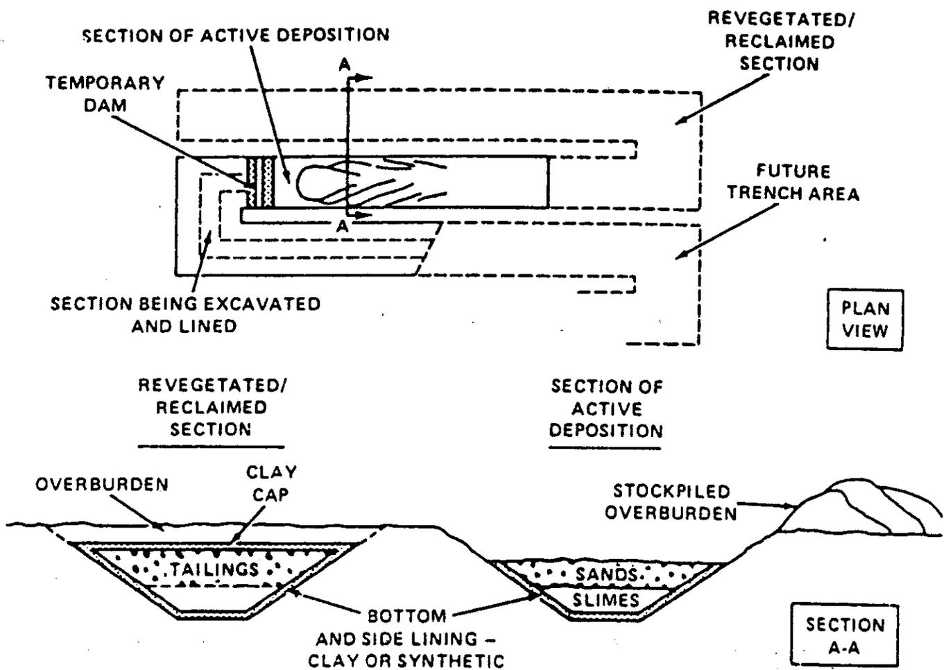
5-16 Disposal in specially excavated below-grade trench. Source: (NRC 1979).
