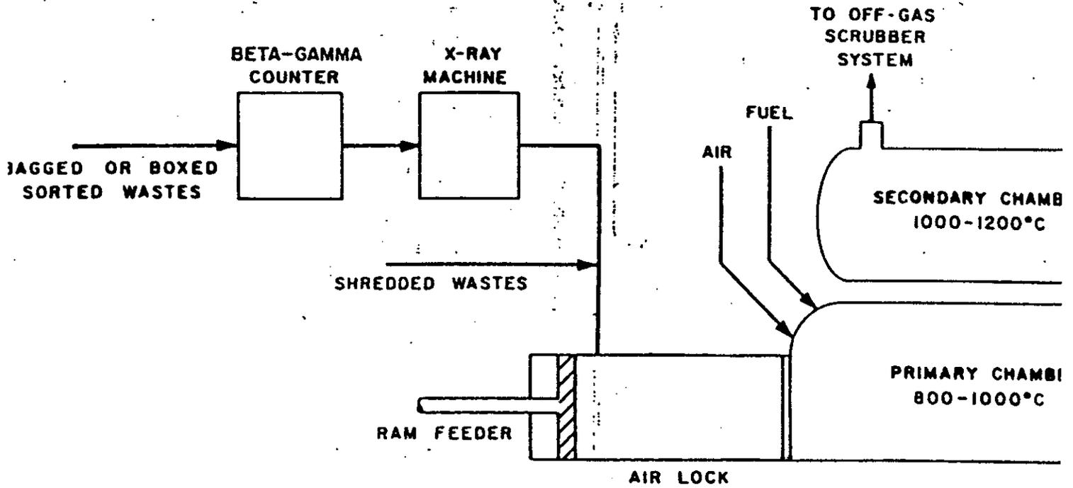
Figure 5-10 Los Alamos National Scientific Laboratory controlled-air incinerator.
