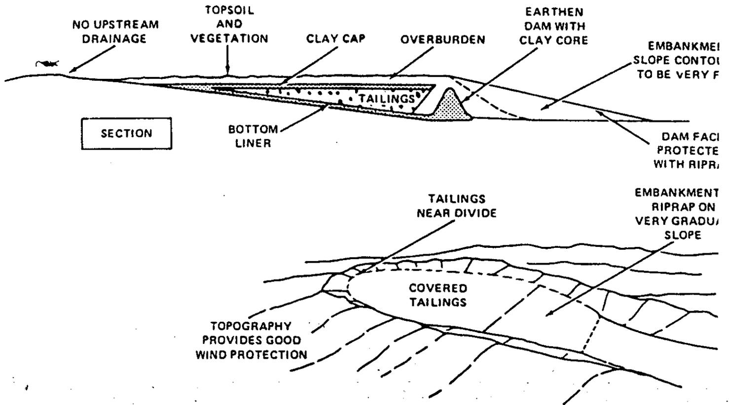
**Figure 6-17** Tailings Disposed above grade with special siting and design featu
