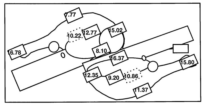
Placement of dosimeters showing dose received in kGy
