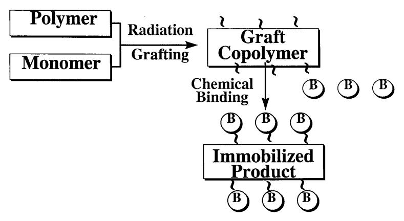
Immobilization of a bioactive component by chemical bonding to a graft copolymer formed by irradiation
