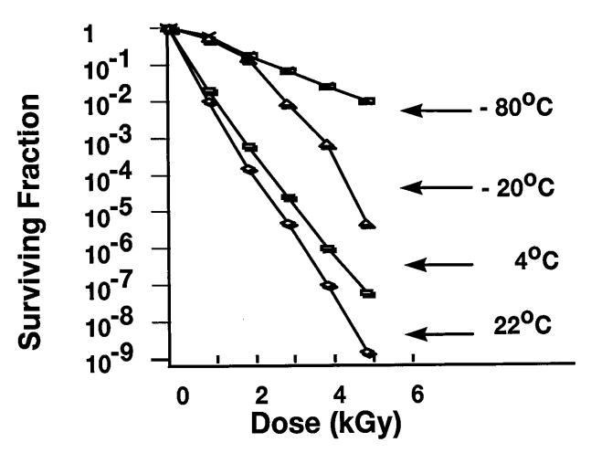
Radiation survival curves for *S.typhimurium*, RIA. The cells were inoculated onto chicken before irradiation (Previte et al., 1970)
