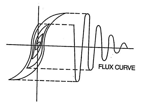
Figure 3.9: Demagnetization
