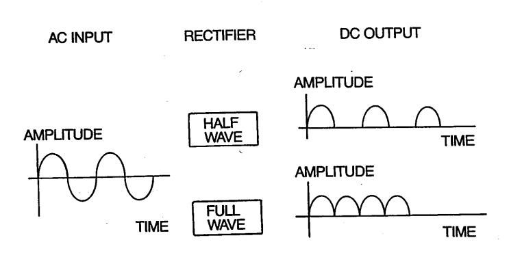
Figure 3.4: Rectified Current
