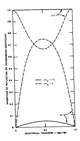
Figure 7.5: Electrical Thickness vs. Reflection and Transmission coefficients
