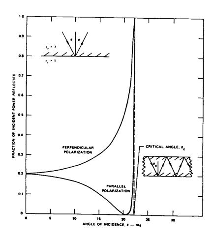
Figure 7.4: Dielectric-to-Air Reflection
