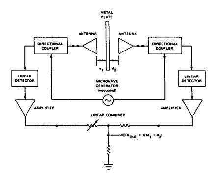
Figure 7.1: Amplitude Method for Thickness Measurement
