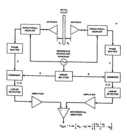
Figure 7.2: Phase-Shift Method for Thickness Measurement
