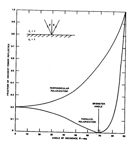
Figure 7.3: Air-to-Dielectric Reflection
