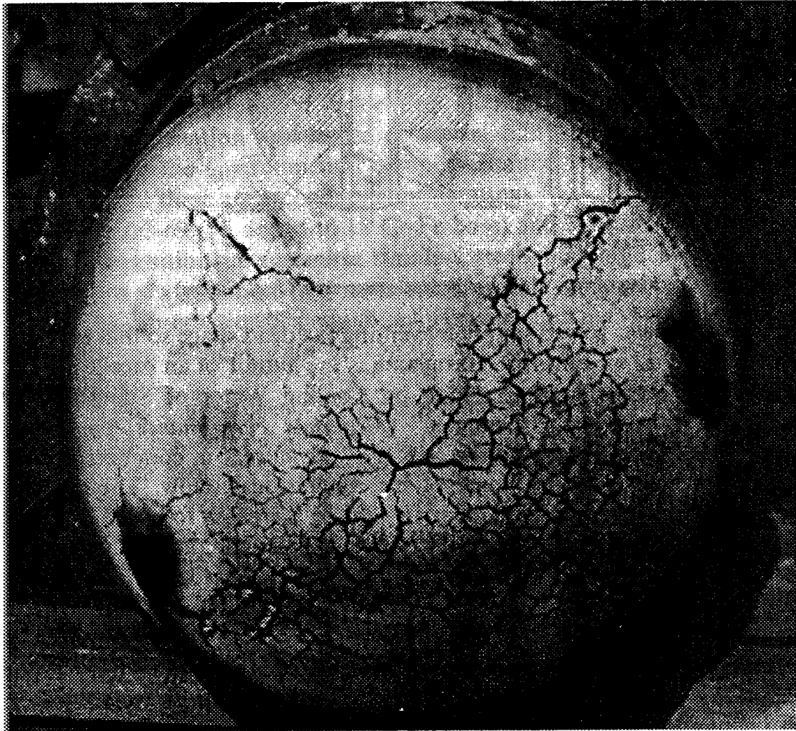
Stress corrosion of type 304 (stainless steel) autoclave. (Mallinckrodt Chemical Works)
