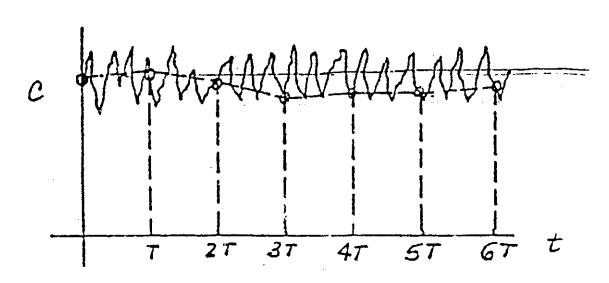
To minimize the effect of aliasing, the sampled signals must be filtered. Virtually all digital control computers provide <u>filter</u> or <u>damping</u> algorithms to reduce the effect of aliasing.
