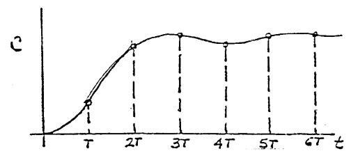
where T is the time interval between samples or sample time. Note that there is loss of information in sampling, namely the response between samples.
