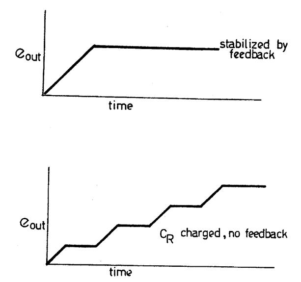
If  $R_p$  is set very large, then the charge time for  $C_R$  will approach infinity and the response will approximate straight proportional control. Reset mode can be considered shut off when  $R_R$  is very large.
