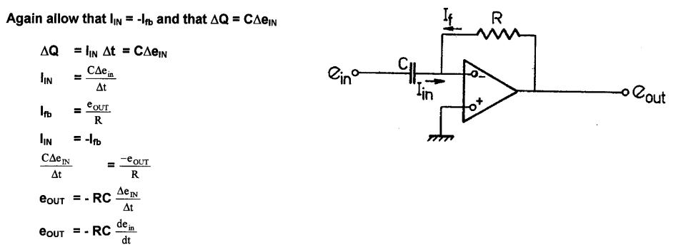
The output voltage is a derivative function of the input signal. All that is required from this development is to know that a derivative function is possible using an OP-AMP with an RC feedback network.
