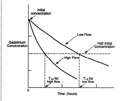
Figure 5.2 Typical Moderator Purification Half Life For Different Purification Flows.
