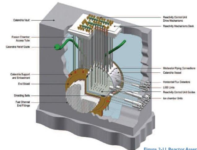
Figure 2-11 Reactor Assembly
