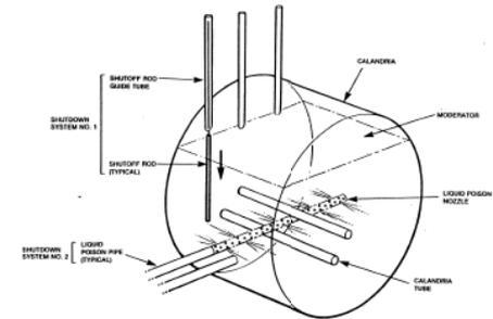
FIGURE 4.3.5 SHUTDOWN SYSTEMS: SHUTOFF RODS AND LIQUID "POISON" INJECTION
