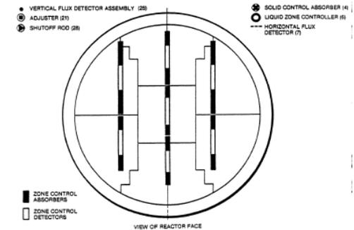
FIGURE 2.4.2 REACTIVITY MECHANISM LAYOUT
