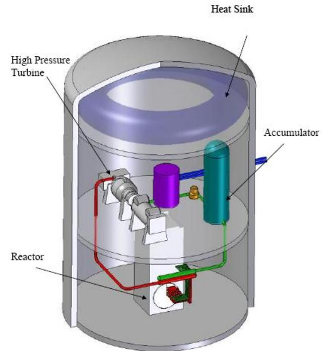
Figure 5: CANDU-SCWR Schematic.
