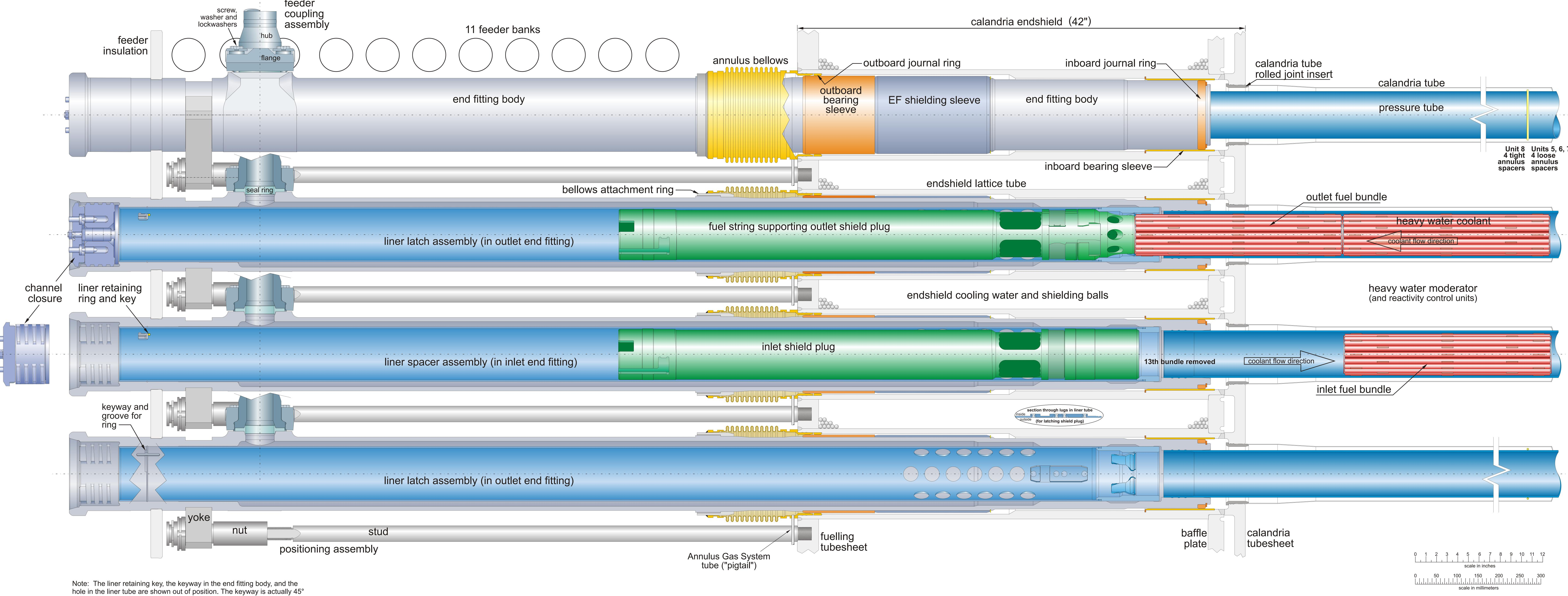
Note: The liner retaining key, the keyway in the end fitting body, and the hole in the liner tube are shown out of position. The keyway is actually 45 to the right of top centre, when looking into the end of the end fitting. Similarly, feeder couplings are generally above center and positioning assemblies below center, oriented to avoid each other.
