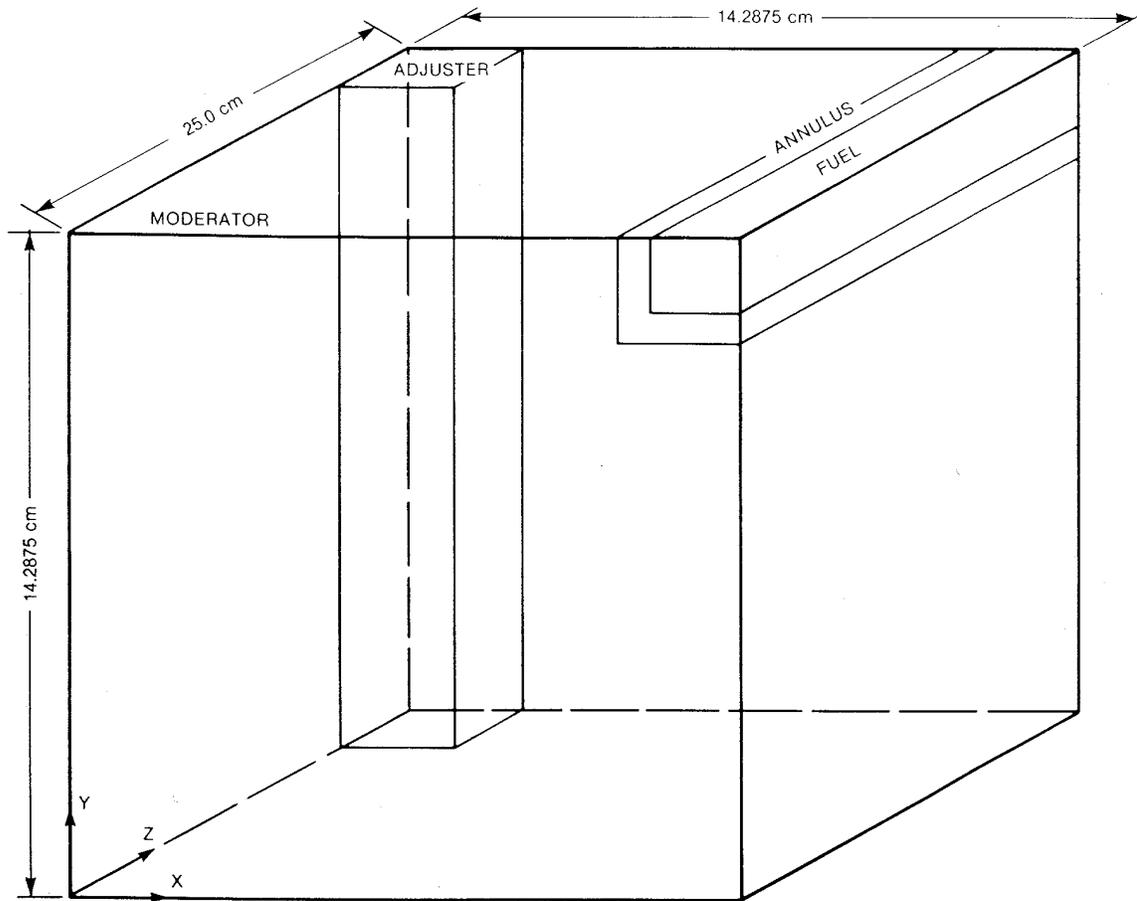
Figure 4.2a Typical RFSP Reactor Model (Face View)
