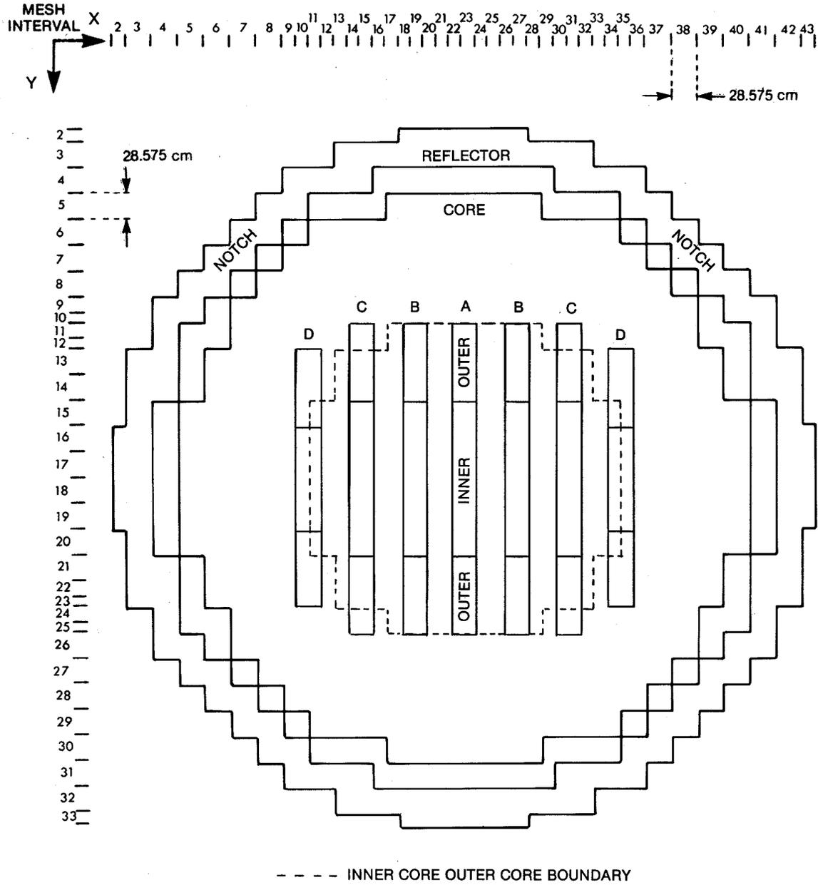
Figure 4.2b Typical RFSP Reactor Model (Top View)
