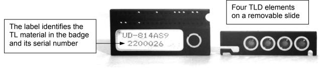
Fig. 6.46. TLD Holder: Rear View
