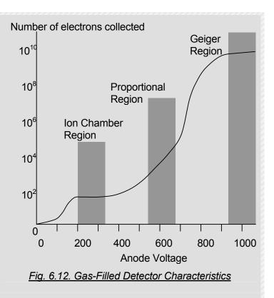
If the voltage is increased much beyond the Geiger region, the breakdown region is reached where continuous arcing occurs across the counter electrodes. This happens because the voltage is high enough to cause ionisation by itself; no initial radiation is needed. Counters must not be operated in the breakdown region, because that's what happens to the detector.
