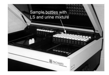
Fig. 6.41. LSC for Bioassay Measurements
