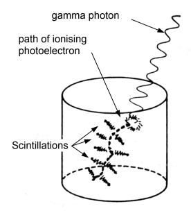
Fig. 6.29. Gamma Absorption in the Phosphor
