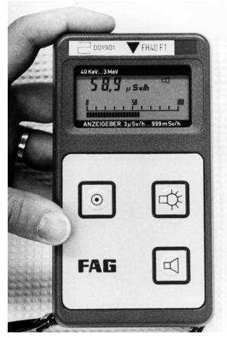
Fig. 6.21. The FAG Gamma Survey Meter with Analogue and Digital Displays
