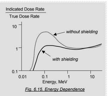
that one of the drawbacks of this is that the shielding has pretty well eliminated the response to low energy photons below 50 keV, because very few of them are now able to reach the tube.
