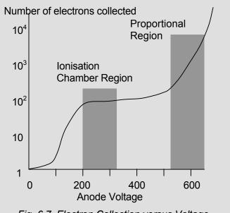
Fig. 6.7. Electron Collection versus Voltage
