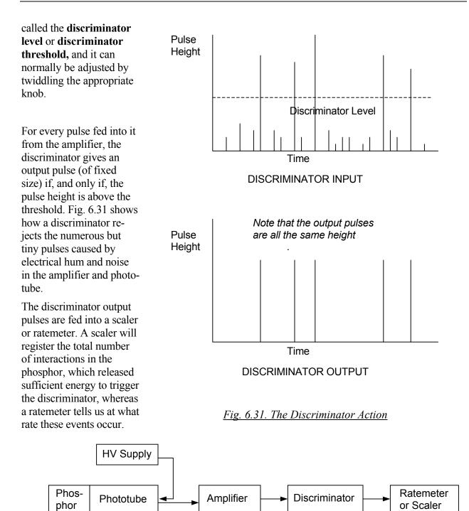
Fig. 6.32. A Complete Scintillation Counter
