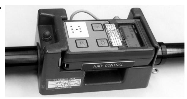
Fig. 6.22. FAG Meter in Telescopic Unit
