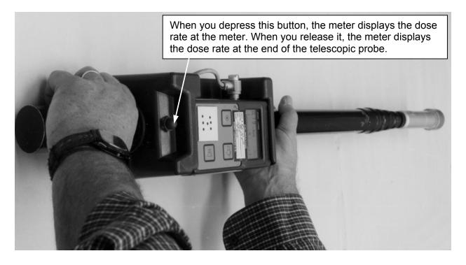
Fig. 6.23. The Telescopic Unit Shown with its Extension
