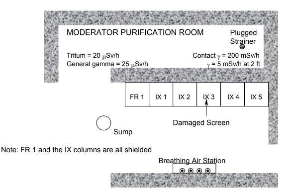
Prepare a work plan to do this. The top of the strainer must be removed and the inside screen must be cleaned of resin. The strainer cannot be completely drained. Gamma and tritium (bubbler) survey results are as shown.
