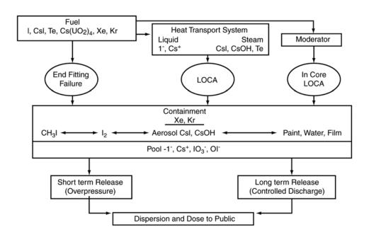
FIGURE 1.1 FISSION PRODUCT BEHAVIOUR UNDER ACCIDENT CONDITIONS
