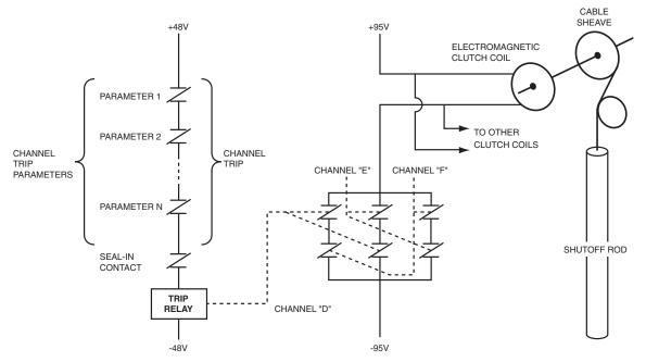
Note: This is a general coincidence circuit - opening of any one contact in each of two channels will trip the reactor
