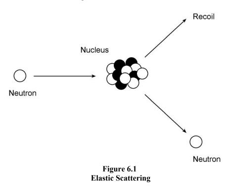
Light nuclei are the most effective for slowing neutrons. A neutron colliding with a heavy nucleus rebounds with little loss of speed and transfers very little energy—rather like firing the cue ball at a cannon ball. On the other hand, neutrons will not be scattered by the light electron clouds surrounding the nucleus, but will travel straight on— much like baseballs through a fog.
