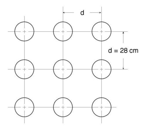
Figure 8.2 Radial Fuel Arrangement
