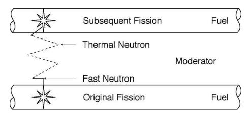
Figure 8.1 Axial Reactor Arrangement
