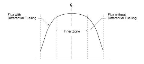
Figure 22.5 Effect of Differential Fuelling
