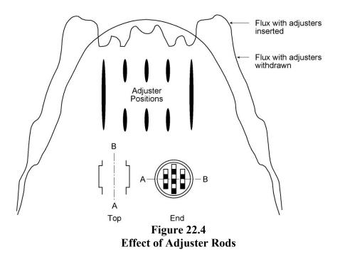
Flux flattening with the use of these rods is quite effective but it does represent a loss in fuel burnup. We accept this because the benefits of increased power production greatly outweigh the higher fuel cost.
