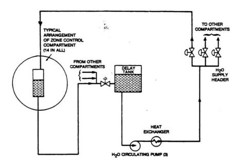
Figure 23.2 Liquid Zone control System (Simplified)
