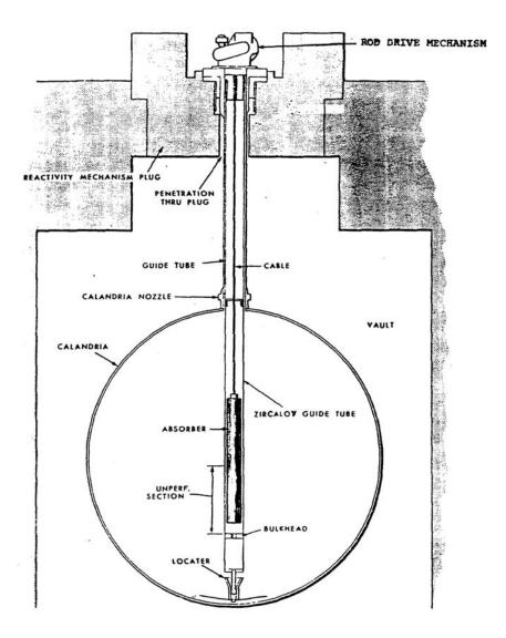
were originally designed to allow some ability to prevent poison outages by removing adjusters from the core as the xenon built up.
