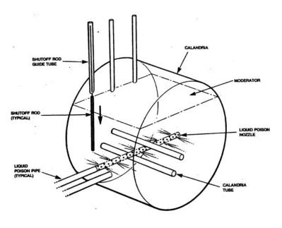
Figure 23.5 Sketch of Shutoff Rods and Liquid Poison Injection
