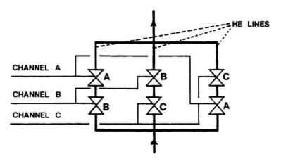
Figure 23.7 Typical Trip Logic
