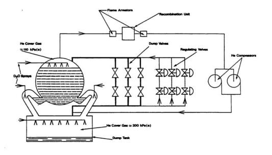
Figure 23.3 Moderator Dump and Level Control at Pickering A
