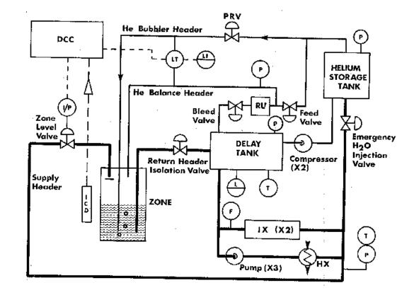
**Figure 5:** Zone Level Control Water and Helium Circuits.
