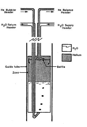
Fig 4: Typical Zone Feed Tube Connections.
