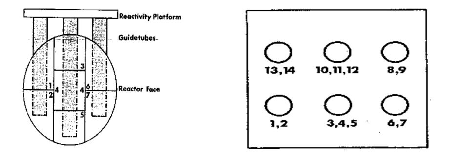
• The reactor face (Figure 2) is marked to show the approximate location of the zones. Each zone is accessible through guide tubes *from the reactivity platform*. It should be noted that the guide tubes can contain either two zones, (e.g., zones 1 and 2), or three zones, (e.g., zones 3, 4 and 5).
