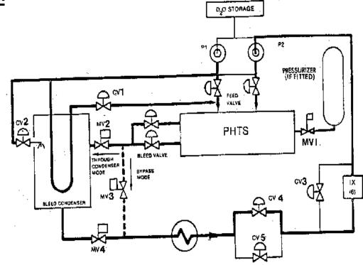
**Figure 5: Overall Control Scheme for HTS.**
