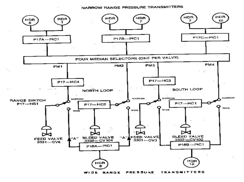
Figure 3: Heat Transport Pressure Control Scheme.
