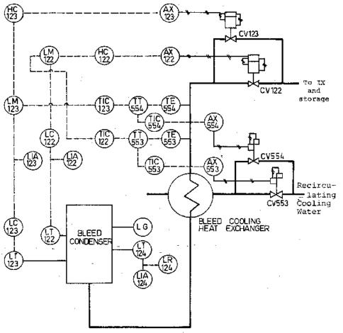
Figure 2: Bleed Condenser Level and Bleed Temperature Control. **Bleed Condenser Level Control (continued)**
