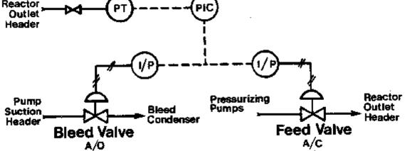
Figure 2: Simplified Split Range Feed and Bleed Control System.
