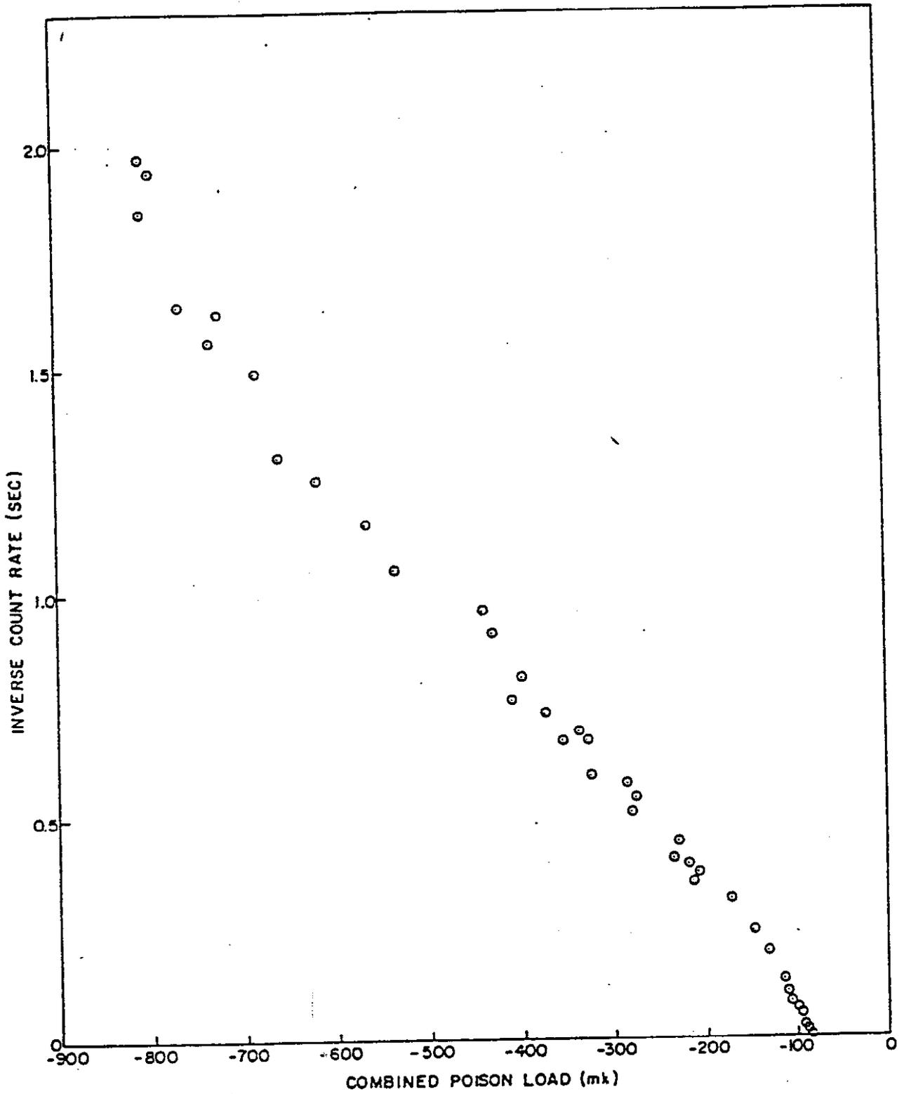
FIGURE 5.2-1 POISON LOAD VS INVERSE COUNT RATE CHANNEL E INCORE BF<sub>3</sub> COUNTER
