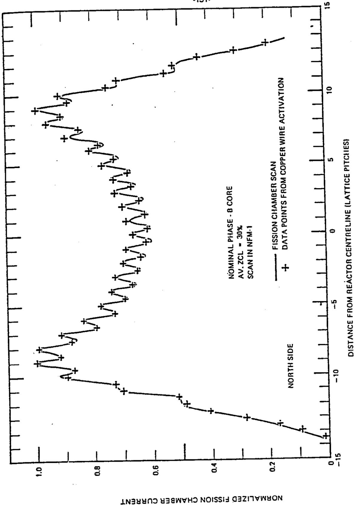
FIGURE 5.2-15 COMPARISON WITH COPPER WIRE ACTIVATION DATA
