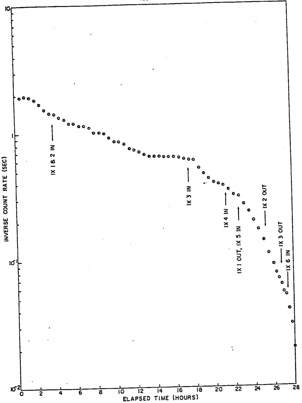
FIGURE 5.2-2 FIRST APPROACH TO CRITICAL CHANNEL D INCORE BF<sub>3</sub> COUNTER
