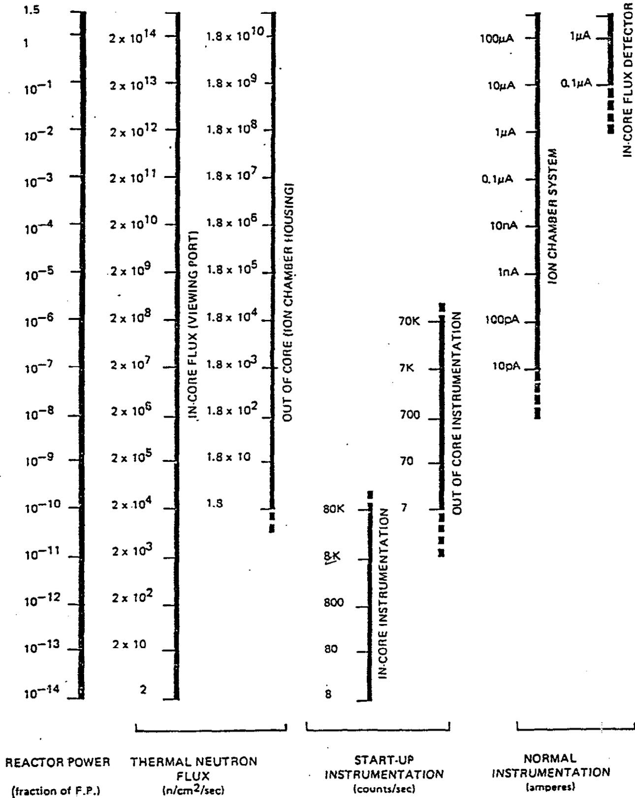
FIGURE 5.2-1.2 RANGE OF SENSITIVITY OF NUCLEAR INSTRUMENTATION FOR REACTOR POWER MEASUREMENT
