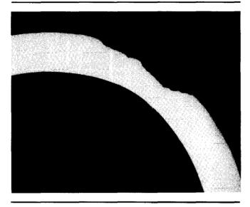
**Figure 4:** Typical deep pit in Incoloy 825 after 26 weeks' exposure to Lake Ontario water (with a crevice).
