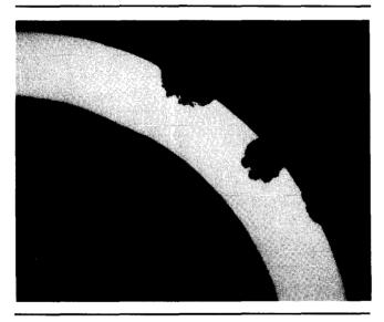
**Figure 5:** Typical deep pits found on AL-6X sample after 26 weeks' exposure to Lake Ontario water (with a crevice).
