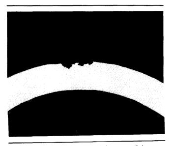
Figure 3: Typical deep pit in Incoloy 800 after two months' exposure to Lake Ontario water (with a crevice).
