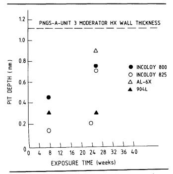
Figure 2: Average maximum pit depths for moderator heat exchanger tube materials subjected to laboratory testing in Lake Ontario water.
