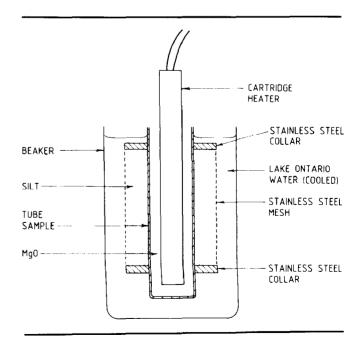
**Figure 1:** Schematic of test apparatus used for corrosion tests with heat transfer and silt crevices. The stainless steel used for collars and mesh was type 304.
