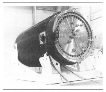
Figure 2: Horizontal testing of the first storage cask (GNs Castor V/21) built by General Nuclear Services.
