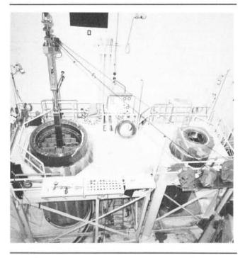
Figure 1: Hot Shop dual-cask work-stand for remote in-air transfer of fuel from shipping casks to storage casks (Spring 1986).
