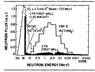
Figure 1: Typical neutron spectra for various nuclear facilities [3].
