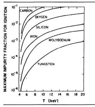
**Figure 7:** Maximum tolerable impurity fraction for ignition of a DT plasma vs. temperature for various impurity species [8].
