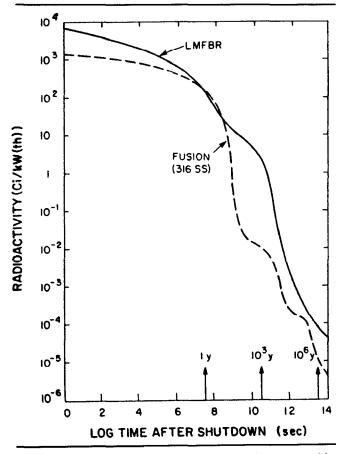
**Figure 3a:** Comparison of radioactive inventory for fission and fusion reactors with SS 316 structure. From: *Hafele W, Holdren JP, Kessler G, Kulcinski GL* Fusion and fast breeder reactors. Austria: Inter. Inst. Applied Systems Analysis, 1977.
