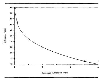
**Figure 5:** Detritiation factor when processing downgraded heavy water. Even small amounts of light water cause a significant drop in the detritiation factor.
