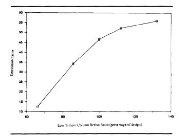
**Figure 4:** The effect of varying the reflux ratio in the first column (Low Tritium Column) in the cryogenic distillation cascade.
