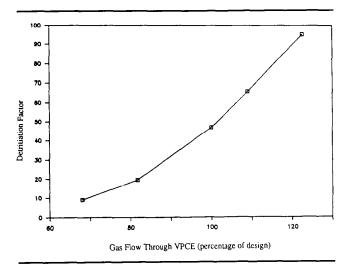
**Figure 3:** Relationship between detritiation factor and deuterium gas flow through the VPCE. The reflux ratio in the first column of the cryogenic distillation (the Low Tritium Column) is assumed to be held constant.
