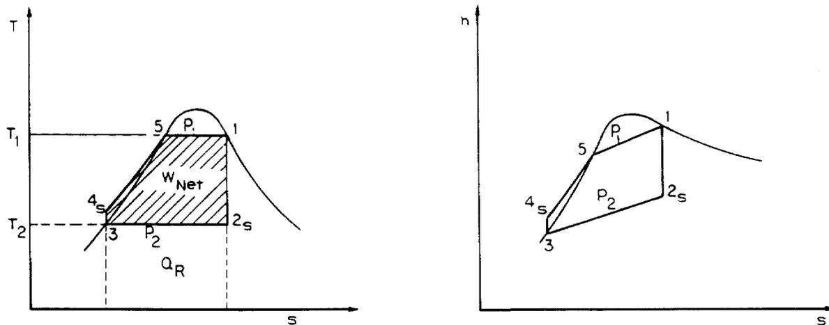
**Figure 4.10** T-s and h-s diagram representations for the ideal Rankin cycles. Note: We are assuming fluid velocities are zero; i.e., the diagram illustrates stagnation properties. [Source: RUS79, figure 2.11]
