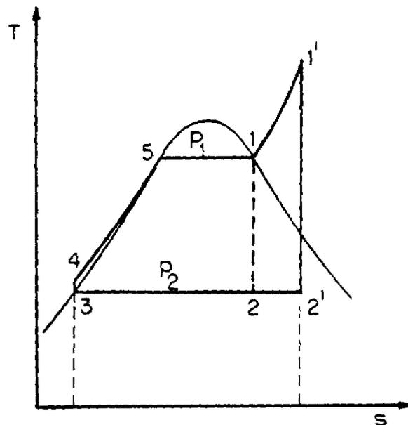
**Figure 4.12** Rankine cycle with superheat [Source: RUS79, figure 2.14]
