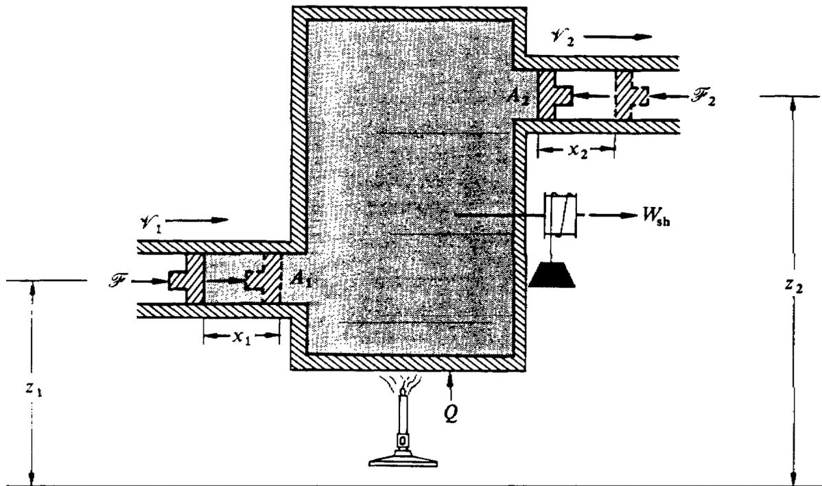
Figure 4.3 Steady flow process [Source: SEA75, figure 3-13]
