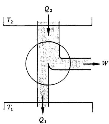
**Figure 4.5** Schematic flow diagram of a heat engine [Source; SEA75, figure 4-7]
