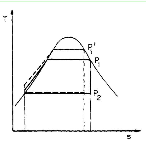
**Figure 4.11** Effects of increasing boiler pressure on the Rankine cycle [Source: RUS79, figure 2.13]
