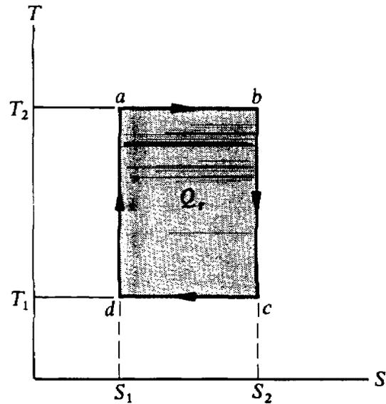
**Figure 4.7** The temperature-entropy diagram for the Carnot cycle [SEA75, figure 5-4]
