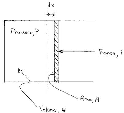
**Figure 4.1** A simple systems for doing work
