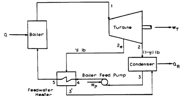
**Figure 4.15** Single heater regenerative cycle [Source: RUS79, figure 2.18]
