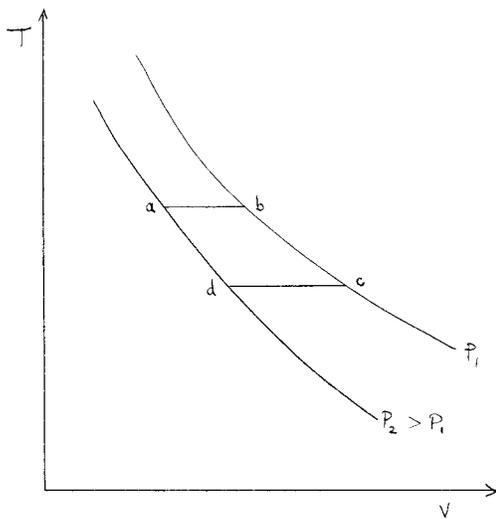
**Figure 4.6** T-v diagram for the Carnot cycle
