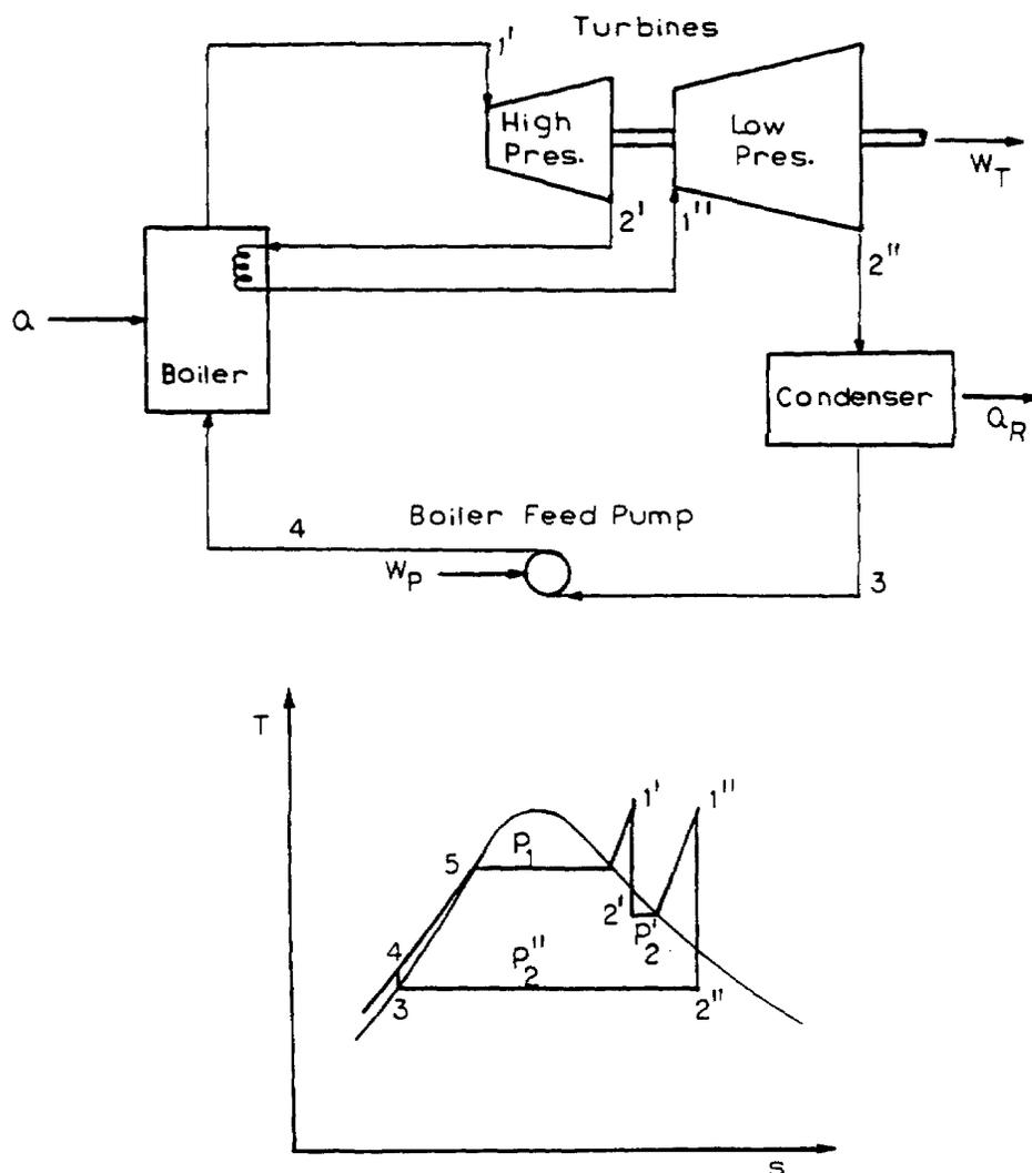
Figure 4.13 Rankin cycle with reheat [Source: RUS79, figure 2.15]
