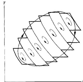
**Figure 4.8** Any arbitrary reversible cyclic process can be approximated by a number of small Carnot cycles. [Source: SEA75, figure 5-3]
