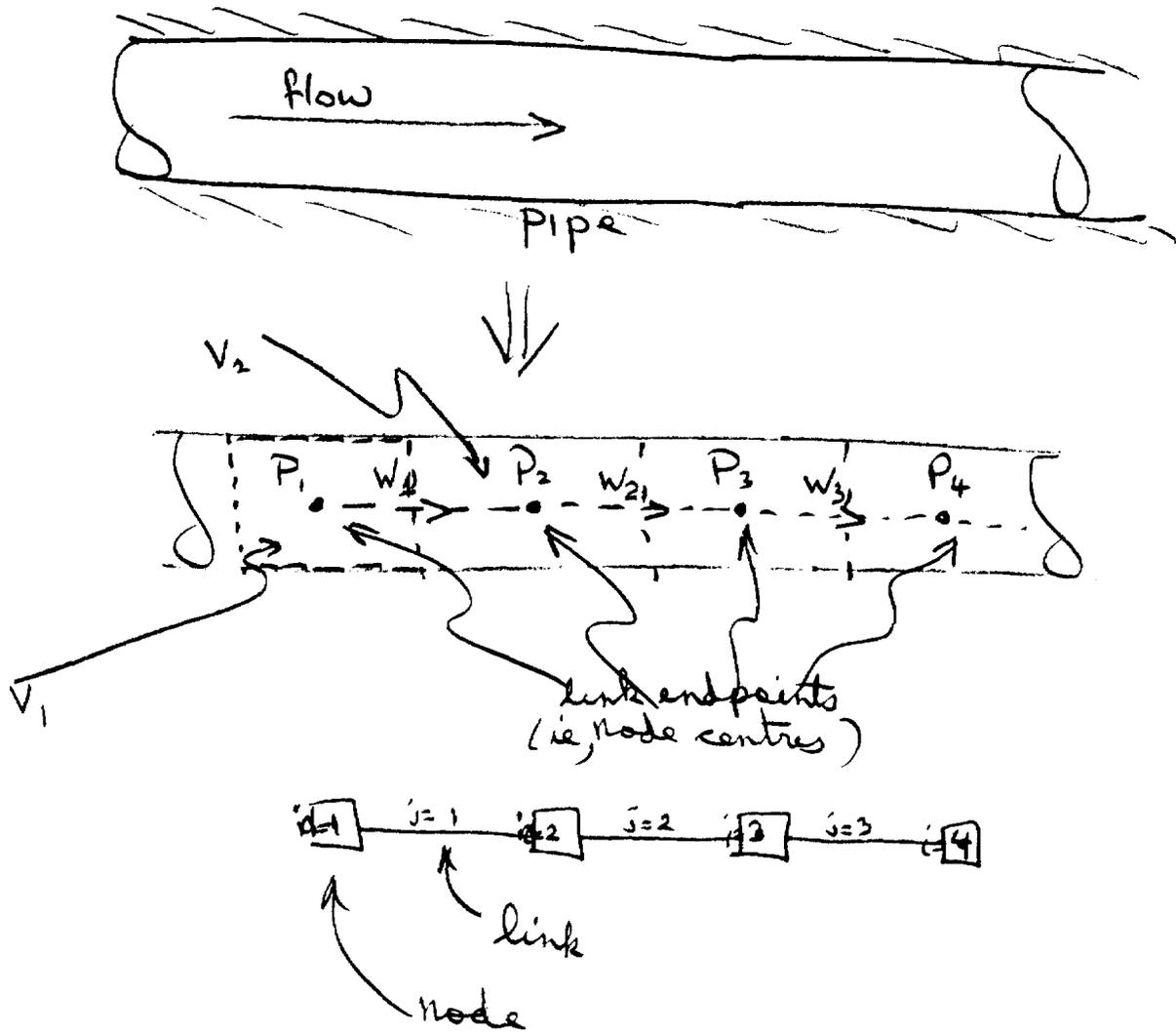
Figure 3.3 Node-link setup for a simple pipe.
